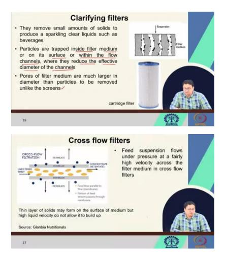
And there we are having higher pressure in one end. That means from that let us say upstream part the suspended solids or slurries are actually being filtered. So the direction is nothing but it is a perpendicular to the membrane surface. Now what is the cross flow? The cross flow is the flow is across.
