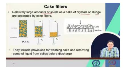
So, there will be a cake formation. So, it will simply block the pores over here on the surface of the filter medium. So, this acts like a, you know, bridge between the particles. So, once it blocks, the other, you know, suspended solids will simply be deposited over one another and eventually it will, you know, form a cake. So, this is called the cake filter or the technique is called cake filtration.
