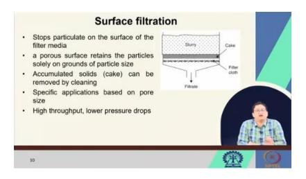
As I was mentioning that it actually arrests all the particles on the surface of the filter media. The porous part actually retains all the particles only on the grounds of particle size. So, if the particles are larger, they will be arrested. Otherwise, it will can pass through. So, that is why you have to wisely choose the kind of what kind of filter cloth or the filter medium we are getting.
