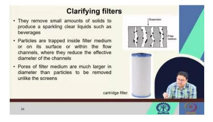
Now, these pores are usually larger than the size of the particle to be removed, the size of the particle to be removed. So, the fluid can easily pass through, and while flowing, the suspended particles will be entrapped within the material, within the filter medium. So, particles are trapped inside the filter medium on its surface or within the flow channels where they reduce the effective diameter of the channels. So, eventually, what does it do? It actually blocks the passages.
