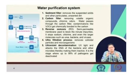
So, if you look at this picture, we have raw water, sorry, raw water. So, in the first two steps, you know, we use a sediment filter and a carbon filter. So, the job of the sediment filter is to remove the large suspended solids and other particles or unwanted dirty material. So, the raw water passes through this sediment filter. So, this is also a filtration process, then it passes to the carbon filter, the activated carbon filter.
