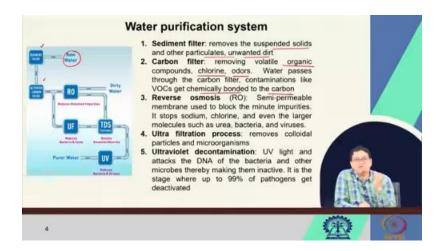
That means the liquid is moving from a lower concentration zone to a higher concentration zone. Reverse osmosis is the opposite of that. So, we apply a very high pressure to the high concentration solution so that we can allow the liquid to pass through the membrane where the solid particles are arrested. So, this is the reverse osmosis process, and the pressure has to be more than the osmotic pressure.
