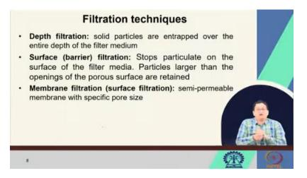
talk about the filtration techniques, broadly they are classified into two. First of all, depth filtration and surface filtration. Another one I have added: membrane filtration. This is also one type of surface filtration technique, but the broad or major categories are these two. The depth filtration and the surface—many times it is called the barrier filtration.
