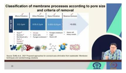
In nanofiltration, sugars, aqueous salts, some multivalent ions, and monovalent ions can be removed. Aqueous salts mean if you take NaCl, table salt, you will have Na+ and Cl- ions. So, you will have the ions, and they can be removed with nanofiltration techniques. Even in reverse osmosis (RO), heavy metals and aqueous salts can also be removed.
