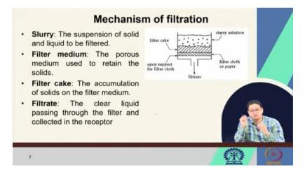
So, here we use a filter medium; many times, the filter medium is also called septum. So, the filter medium is the very essential and core part, ok. Here we have the suspended solution or the slurry. So, this one has got some solid particles.
