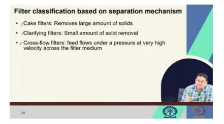
This process is also called the cake filtration technique. Clarifying filters actually remove a small amount of particles. In the cross-flow filters, feed flows under pressure at a very high velocity across the filter medium. Let us look at it. Let us look at some pictures; then we will have a better idea, okay?
