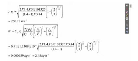
So, which can be correlated with this can be a little You see that 0.00689 kg per second that we have converted into 2.48 kg per hour, right. So, this we are also not going to check because we have already done with the velocity. Now, maximum velocity for maximum velocity, we have said that the pressure ratio is 0.528.
