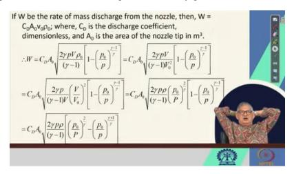
Into  $P_0$  by P to the power 2 by gamma minus  $P_0$  by P to the power gamma plus 1 by gamma, right. This we have developed, right. Then we also have developed this: if we differentiate W, that is discharge rate, with respect to  $P_0$ , right. Then we get dW / dP<sub>0</sub>, and it is a complex one which has come up like  $C_D A_0$  under root 2 gamma P rho by gamma minus 1 d dP<sub>0</sub> under root
