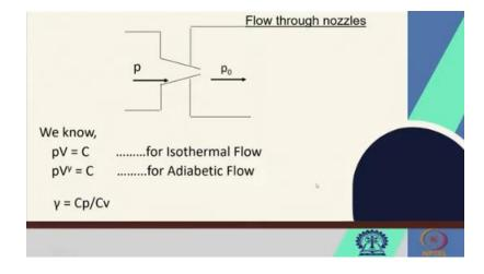
And we also said that the flow is more adiabatic than isothermal. Because temperature may change. I had given an example also that in the refrigeration cycle, in the vapor compression refrigeration cycle, the fluid or liquid refrigerant flows through a valve that is called an expansion valve. When it goes through that from a very high pressure to a very low pressure, there is a change in the fluid, and this change is called
