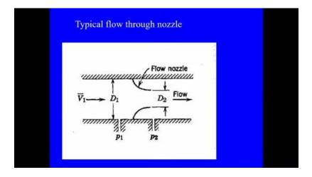
Inside pressure  $P_1$  is high, and outside pressure  $P_2$  depends on the value of  $D_2$ , right. So, this is how it can be measured experimentally. So, this is another typical function of a nozzle. So, there are many nozzles that are blown with air, right, or it could be some fluid. So, droplets filled with tiny air bubbles are blown.
