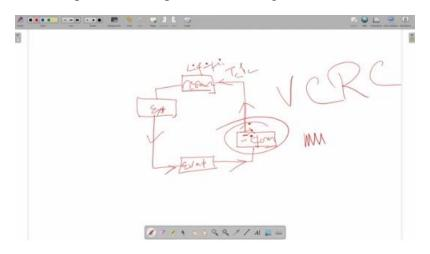
Change in temperature, a drop from  $T_c$  to  $T_e$ , happens, and it is definitely a drastic drop a lot of temperature drop depending on what your evaporator temperature requirement is, right. Then we come to this point, okay. We have shown you that in the refrigeration cycle, from high pressure to low pressure, fluid is moving, right. And there, we have just shown that the temperature is being dropped drastically.
