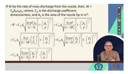
How that also is shown, but still how W is equal to  $C_D A_o v_o$  rho<sub>o</sub>, right?  $C_D$  is dimensionless. But  $A_o$  is meter squared, vo is meter per second, and rhoo is kg per meter cubed, right? So, this meter squared, this meter, and this meter cubed cancel out, resulting in kg per second, which is W. Right. So, we can say that the discharge rate, right, discharge rate is W equal to  $C_D A_o$  under root 2 gamma P rho by gamma minus 1.
