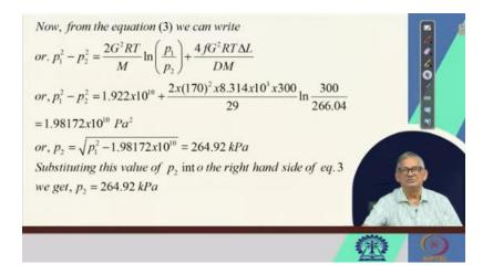
Root means the solution of the equation, ok. So, here our first approximation, as we said, is We have taken the previous value, obtained value of  $P_2$ , that is 266.04. By that, we get  $P_1$  square minus  $P_2$  square is equal to 1.98172 into 10 to the power 10 Pascal square, right. Therefore,  $P_2$  can be obtained.
