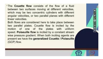
Both flows are considered here to take place between two parallel plates. Couette flow is incited by the motion of the one of the plates with uniform speed. Poiseuille flow is incited by constant stream wise pressure gradient. When both inciting agents are present, we have the generalized Couette / Poiseuille, that is, GCP flow. Right?
