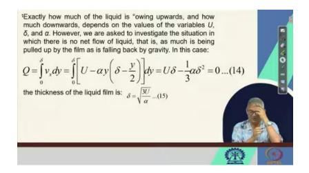
flowing upward like this and some liquid is flowing downward like this right. Then the question is how much liquid is flowing upward and how much liquid is flowing downwards right. So, this depends on the values of the variables that is u, del and alpha. However, we are asked to investigate the situation in which there is no net flow of liquid that is as much as being pulled up by the film as is falling back by gravity.
