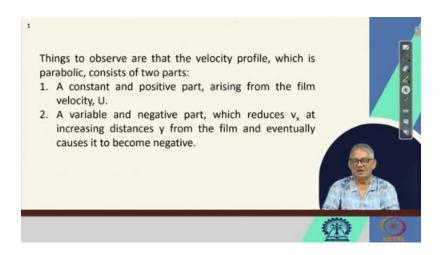
One is positive arising from the film velocity u. and the other one is slightly negative and this reduces  $v_x$  at increasing distance of y from the film and eventually causes it to become negative, right? So, this tells like this, okay? If you plot it, you see. This is the delta, ok.
