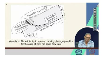
So, with this note let us now proceed for the next. What is that? That this is velocity profile in thin liquid layer on moving photographic film for the case of zero and net liquid flow rate. Now, if we look at exactly how much of the liquid is flowing upwards and how much downwards. We have just seen some liquids are
