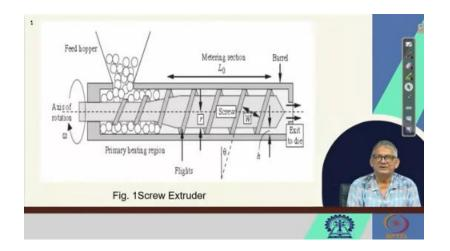
The polymer typically enters the feed hopper as plates and is pushed forward by the screw which rotates at an angular velocity omega. Clockwise it is seen by an observer. along the axis from the inlet to the exit. Yeah, why I am giving so much emphasis on this because this is also telling a process. Yeah, which obviously is related to the flow of the fluid, but keep in mind
