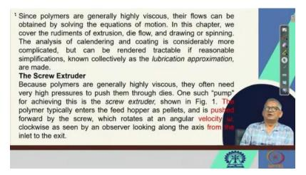
If we look into that screw extruder, yeah there could be single screw, there could be twin screw like that many. So, because the polymers are generally highly viscous, they often need very high pressure to push. them through dies. One such pump for achieving this is the screw extruder. This is shown as in the next figure.
