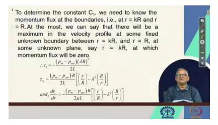
So, we cannot say that at r is equal to R, at r is equal to kR and at r is equal to capital R, the boundary will be like this. So, we can say that there will be a maximum in the velocity profile at some fixed point, which is unknown, and beyond the normal boundary between r is equal to kR and r is equal to R. Obviously, it has to remain within that annular space. So, it should be between r is equal to kR and r is equal to kR
