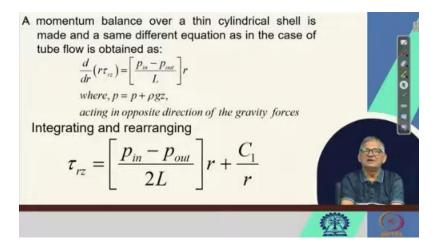
Here, capital P is P plus rho  $g_z$  because, if you remember from the pictorial view, we said that the fluid is flowing from the bottom to the top, right. So, we have the pressure difference, okay, that is P. That actual pressure is this P plus rho  $g_z$ , which is the height of the cylinder column, whatever you call it. So, that is capital P is P plus rho  $g_z$ . Now, this acts in the opposite direction of the gravitational forces, definitely, right.
