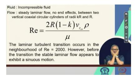
So, what do we do now? We take a momentum balance over a thin cylindrical shell and make the momentum balance. And the same differential equation as in the case of tube
