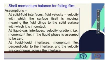
This means the fluid clings to the solid surface with which it is in contact. Right? At liquidgas interfaces, which I have shown you and I told you that you remember. At liquid-gas interfaces, this is that, unless I take some pen it will not be.
