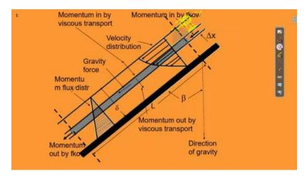
Now, we need to know the boundaries again. At x equals to 0,  $tau_{xz}$  is also equal to 0. At x is equal to x, at x equal to 0, tauxz is 0. So, C<sub>1</sub> is also 0 and therefore, we can write  $tau_{xz}$  is rho  $g_x$  into x cos beta and del Ok, we define  $tau_{zz}$  as no, this  $tau_{zx}$  only, not z is mu minus mu del vz / del x and this is equal to rho  $g_x$  into x into cos beta.
