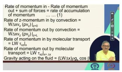
It is the rate of momentum out by convection. Then, once convection is over, it becomes molecular transport, that is, the rate of momentum in by molecular transport is L w tauxz at x. And the rate of momentum out by molecular transport is Lw tau<sub>xz</sub> at x plus delta x. Gravity acting on the fluid is Lw delta x into rho  $g_x$  cos beta. Lw delta x is the volume element. Rho  $g_x$  is the
