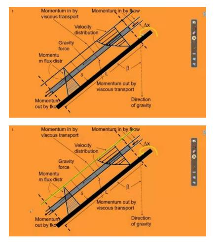
This is the direction of gravity. This is the direction of gravity, and the angle between the surface and the vertical is angle beta, right? The length, or thickness, whatever you call it,
