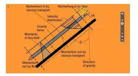
So, that means if that is the truth, then we can say that At x equals to 0, the boundary is tauxz is equal to 0, that was our, this is in accordance with the assumptions we have made, right. Then if delta x tends to 0, tauxz del x is equal to rho  $g_x$  cos beta. So, again on integration, this gives tauxz is equal to rho  $g_x$  x cos beta plus C<sub>1</sub>. So, the C<sub>1</sub> is the integration constant.
