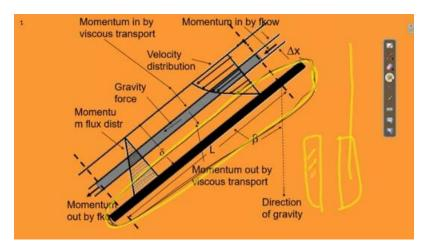
So, the gap between them is very, very narrow. So, a drop of slurry falls here, which gradually gets vaporized, and you get a concentrated outlet. Right? This we have shown, we have said in the beginning, right? Now, we have taken it inclined because we get cos beta, the angle of inclination, right?
