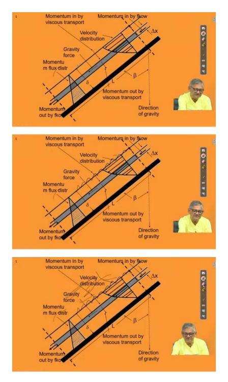
At liquid-liquid interfaces, momentum flux perpendicular to the interface and the velocity are continuous across the interface, right. With these three assumptions, if you want, you can repeat quickly that at solid-fluid interfaces, that is the bottom part Velocity, fluid velocity is the velocity with which the surface itself is moving, meaning the fluid clings to the solid surface with which it is in contact, right? And at liquid-gas interfaces, the velocity
