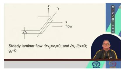
There are two directions, which are z and x. The flow is happening through the x direction, right? The gap between the two plates is 2  $z_0$ , as it is said, right? The third dimension is y. Okay, then, at steady laminar flow, obviously,  $v_y$  and  $v_z$  are 0.  $v_x$  cannot be 0 because, if  $v_x$  is 0, then there will be no flow. So,  $v_y$  and  $v_z$  are 0, and del  $v_x$  / del x is also 0. Since it is horizontal, we can say that the value of g or g at x is also equal to 0, right?
