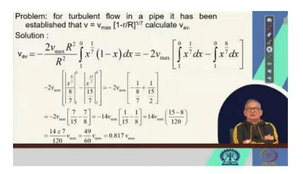
So, that you can find out very easily by substituting 1 minus r by R as dx or x rather, right. So, you can find out what the value of dx is and what the value of dr is accordingly. So, on integration, you get that equals to minus 2  $v_{max}$  into rather it equals minus 2  $v_{max}$  between 0 1 to 0 x to the power of 1 by 7 dx minus 1 to 0 x to the power of 8 by 7 that is 1 minus 1 by 7.
