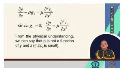
Now, del p / del x being equal to mu del 2  $v_x$  / del x square and equals to constant on integration, we get On integration and using the boundary condition, then we get del  $v_x$  del x, del  $v_x$  / del z is equal to 0. You look at here, it was del  $v_x$  / del x is equal to 0, and now we are saying that del  $v_x$  / del z. This is the boundary condition. del  $v_x$  / del z is equal to 0 again at z is equal to 0, right? Because, it is symmetrical.
