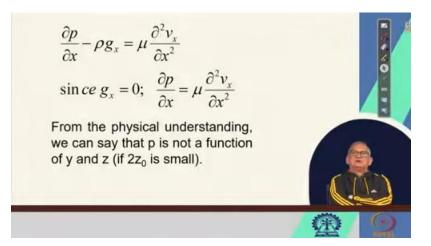
So, del P / del x minus rho  $g_x$  is equal to mu del 2  $v_x$  / del x square, and since  $g_x$  is 0, del P / del x is mu del 2  $v_x$  del x square, right? So, already, we have said from the physical understanding that we can say P is not a function of y or z. If 2 z is small, if 2 z is big, then it may not be, but if 2 z or 2  $z_0$  is small, then p is not a function of both y and z.
