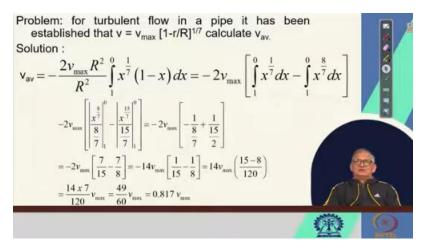
Now, what we have made x to the power of 1 by 7 or x rather, that we have made by substituting the value of 1 minus r by R, right? So, that is 1 minus r by R to the power of 1 by 7. And if you take that 1 minus r by R is equal to x and you see your limit that is 0 to r. That is changed to 1 to 0, right?
