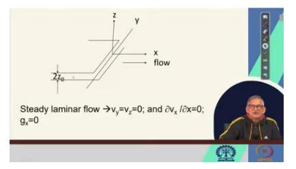
What is the boundary? At z is equal to 0? No, at z is equal to  $z_0$ , right? At z is equal to  $z_0$ , it could be plus  $z_0$ , or it could be minus  $z_0$ . If this is plus  $z_0$ , then this is minus  $z_0$ , right. So, at both z is equal to plus minus  $z_0$  at the center, we can say  $v_x$  is equal to 0, because this is the inner surface. This is also the inner surface at z is equal to  $z_0$  or z is equal to minus  $z_0$ .
