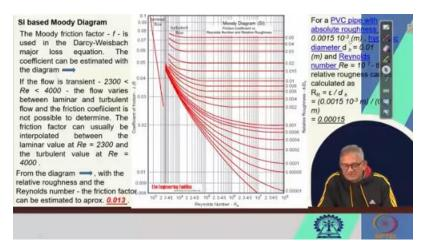
The flow varies between laminar and turbulent flow, and the frictional coefficient is not possible to determine. The friction factor can or usually be interpreted between the laminar value that is somewhere at less than 2300, and the turbulent value, which is somewhere at more than 4000 Reynolds number, right. Then, from the diagram with the relative roughness and the Reynolds number, the frictional factor can be estimated, right.
