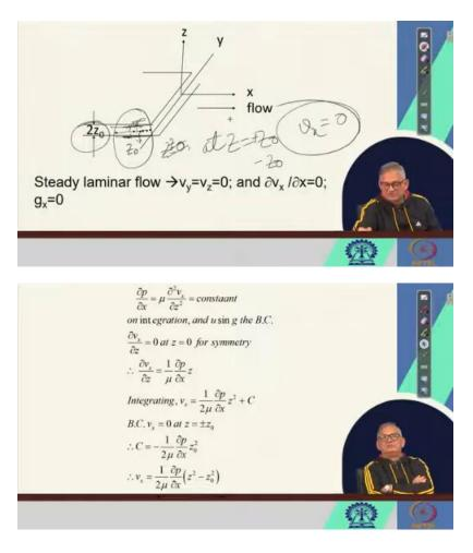
Therefore,  $v_x$  can be rewritten as. 1 by 2 mu del P del x into z square minus  $z_0$  square, right? So, this is what we have found out when two flat parallel plates are present, a flow of fluid is happening through that, and we said the flow is laminar. We also said not only is the flow laminar, but we also said that the density is constant, right? And the gap between the two is 2  $z_0$ , right? The gap between the two is 2  $z_0$ .
