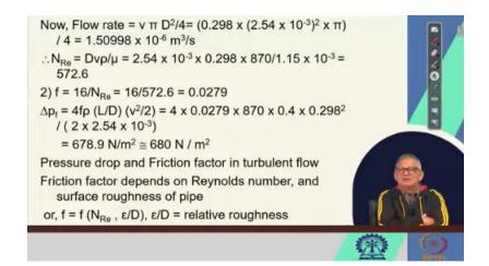
So, there the flow or roughness is very, very high. So, like that, depending on the roughness of the pipe, the friction factor, when we consider it to be turbulent, then the drop of the friction factor is related to Reynolds number as well as the roughness of the pipe. Or surface roughness of the pipe. This was again highlighted by some very renowned scientist, right. So, we call him definitely a pathfinder.
