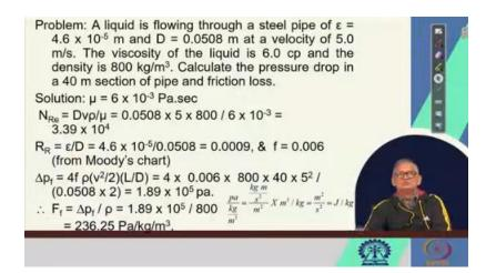
Then, calculate the pressure drop in a 40-meter section of pipe and the frictional loss. I repeat, a liquid is flowing through a steel pipe. Again, here you see the pipe has been said to be made of steel, right. So, it has an epsilon, which is 4.6 into 10 to the power of minus 5 meters, and D is 0.0508 meters. at a velocity of 5 meters per second.
