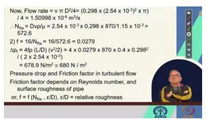
v is 0.298 into 2.54 10 to the power minus 3 whole square, that is so much D square into pi by 4, this is equal to 1.50998 10 to the power minus 6 meter cube per second. You can do a cross check again with your calculator and see whether it is coming, the flow rate to be 1.50998 into 10 to the minus 6 meter cube per second or not, hopefully it should come. Therefore, we can write that the Reynolds
