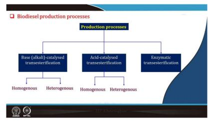
Then biodiesel production processes are base (alkali)-catalyzed transesterification, acidcatalyzed transesterification, or enzymatic transesterification. Both acid and alkali catalyzed transesterification can be homogeneous or heterogeneous.
