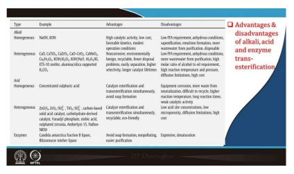
This are the some of the examples of different types of alkali-catalyst, homogeneous and heterogeneous, acid-catalyst and enzymes. So, you have seen that is, advantages of the homogeneous alkali-catalyst include high catalytic activity, low cost, favorable kinetics, and modest operation conditions. Disadvantages are low free fatty acid requirement, anhydrous conditions, saponification, emulsion formation, more wastewater from purification etcetera.
