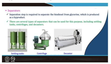
Then after the reactor, it is passed through the separators to separate the biodiesel from the glycerine. There are several types of separators that can be used for this purpose including settling tanks, centrifuges, or the decanters.
