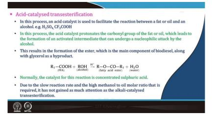
Acid-catalyzed reaction is used in sulphuric acid or trifluoroaceticacids. In this process, the acid catalysts protonates the carbonyl group of the fat or oil, which leads to the formation of an activated intermediate that can undergo a nucleophilic attack by the alcohol. This results in the formation of ester, which is the main component of biodiesel
