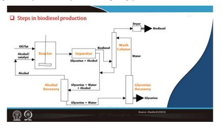
Steps in biodiesel production. It was reported by Dunford in 2023 recently, that is, the oil and fat it is fed into the reactor and then alcohol as a catalyst they are fed into the reactor and here the reaction takes place, fatty acid methyl ester is formed then they are passed through the separator where glycerine and alcohol are separated. The glycerine portion may come contain some water plus alcohol as well. So, this is sent for alcohol recovery
