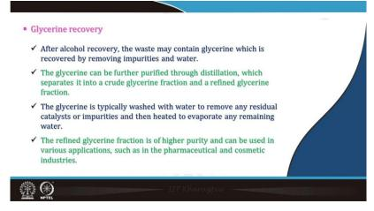
Then glycerine recovery, that is after alcohol recovery the waste may contain glycerine, which is recovered by removing impurities and water. The glycerine can be further purified through distillation, which separates it into a crude glycerine fraction and refined glycerine fraction. The glycerine is typically washed with water to remove any residual catalysts or impurities and then heated to evaporate any remaining water. The refined
