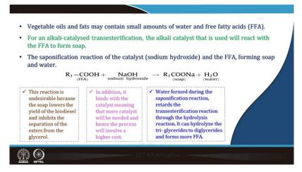
Vegetable oils and fats may contain a small amount of water and free fatty acids. For an alkali catalyzed transesterification, the alkali catalyst that is used will react with FFA to form the soap. The saponification reaction of the catalyst and the FFA form the soap and water.
