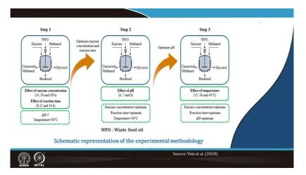
There are three step processes given by Veda et al. in 2020. They gave schematic representation of the experimental methodology to have this process and they studied the effect of enzyme concentration like 14, 16 and 18 percent concentration, effects of reaction time in step 1, pH was 7 and temperature 38 degree Celsius.
