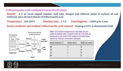
Trifluoroacetic acid-catalyzed transesterification, here a 4 ml screw-capped stainless-steel tube is charged with the different moles of soybean oil and methanol, and a desired amount of trifluoroacetic acid. Temperature is generally 100 to 200 degree Celsius. Reaction time may be 1 to 4 hours. Centrifugation is given to 12000 g for 5 minutes and excess methanol and residual trifluoroacetic acids removed by heating at 65 degree Celsius in thermostatic baths.
