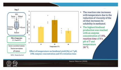
Then in third step, there is the effect of temperature 35, 38 and 40 degree Celsius and you can see here the reaction rate increases with temperature due to the reduction of viscosity of the oil that increases its solubility in methanol. The highest biodiesel production was reached with an enzyme concentration of 14 percent, reaction time of 8 hours, pH 7, and temperature 38 degree Celsius that gives around 90 percent biodiesel yield.
