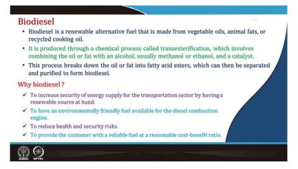
Biodiesel is a renewable alternative fuel that is made from vegetable oils, animal fats or recycled cooking oil. It is produced through a chemical process called transesterification, which involves combining oil or fat with an alcohol usually methanol or ethanol as a catalyst. This process breaks down the oil or fat into fatty acid esters, which can then be separated and purified to form biodiesel.
