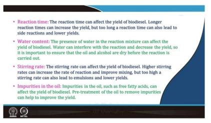
Reaction time can increase the yield, but too long a reaction time can also lead to side reactions and lower yields. The presence of water in the reaction mixture can affect the
