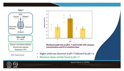
Similarly, that is you see, the higher yield was obtained at pH 7. When the effect of pH 6, pH 7, and it was at pH 7, the highest yield was obtained in comparison to pH 6 and pH 8. So, maximum lipase activity was found at pH 7.
