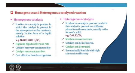
Heterogeneous catalysis, it refers to a catalytic process in which the catalyst is present in a different phase than that of the reactants and usually it is in the solid phase like calcium oxide, potassium carbonate etc. It has a medium conversion rate, catalyst can be recovered here. However, catalyst accordingly therefore, catalyst can be reused and it is an economically feasible with high conversion efficiency.
