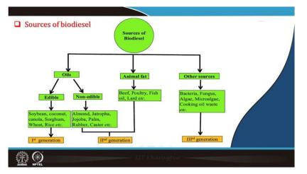
Sources of biodiesel include that is oils, animal fats, or other sources. In the oils, it may be edible oil like soybean, coconut, canola, sorghum, etc., they are considered the firstgeneration oil sources. Whereas, the second-generation oils include non-edible oils like
