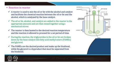
Then in the reactor which you have seen, that is, where alcohol and these reactants they are used. So, the reactor is used to mix the oil or fat with the alcohol and the catalyst to
