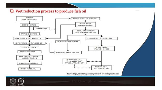
Then wet reduction process to produce fish oil in this slide is shown that is raw material it is cooked, then drained pressed and the drainings are there that is pressed liquid is solids removal and then it is oil and water separation you get a stick water and which is evaporated and different drying stages you get and finally, you get fish meal and after this pressing in different operations you get various fish oil ok.
