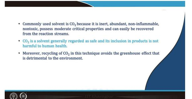
A commonly used solvent is  $CO_2$  because it is inert, abundant, non-inflammable, nontoxic, possesses moderate critical properties, and can easily be recovered from the reaction streams.  $CO_2$  is a solvent generally regarded as safe and its inclusion in products is not harmful to human health. Moreover, recycling  $CO_2$  in this technique avoids the greenhouse effect that is detrimental to the environment.
