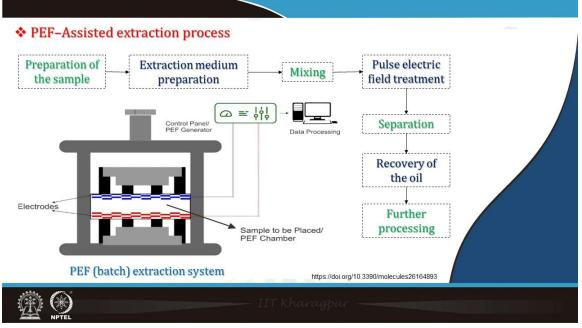
This is the PEF-assisted system where these are the electrodes and in between electrodes, the sample is placed. So, it needs first preparation of the sample, then extraction medium preparation, mixing, then pulse electric field treatment, separation, recovery of the oil, and then further processing. So, just after PEF treatment, it can be further subjected to the extraction process either by solvent extraction or by any other methods. So, PEF increases the pores.
