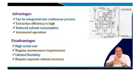
The advantage of this system include that it can be integrated into a continuous process extraction efficiency. In this system is high, there is a reduced solvent consumption and again it is automated operation. However, the disadvantages are the high initial cost, regular maintenance requirement, limited flexibility and also requires a separate solvent recovery system.
