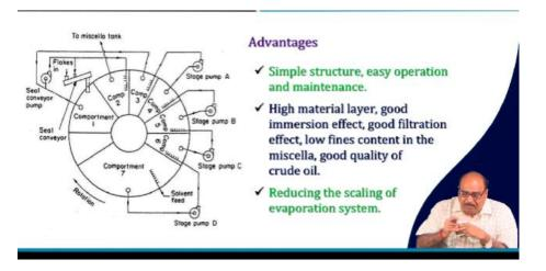
The advantage is it is simple structure, it has easy operation and maintenance, high material layer, good immersion effect, good filtration effect, low fines content in the miscella, very good quality of crude oil can be obtained and the reducing and scaling of the evaporation system is another advantage of this process.
