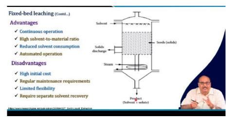
So, this is you can say the fixed bed leaching system here that is the here there is solid sheet solids are there and then it improves solvent is coming. So, it basically the it is the in this the solvent oils are getting dissolved into the solvent and finally, we get the miscella is recovered from the product. So, this system has both again like any system advantages and
