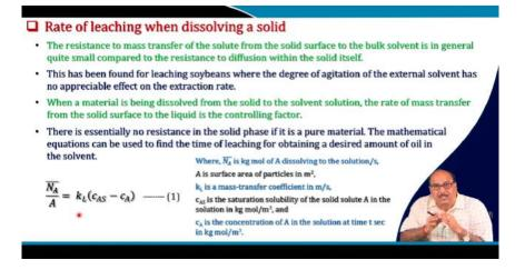
So, rate of leaching when dissolving a solid is very important. The resistance to mass transfer of the solute from the surface of the solid to the bulk solvent is in general quite small compared to the resistance to diffusion within the solid itself. This has been found for leaching soybeans where the degree of agitation to the external solvent has no appreciable effect on the extraction rate. When a material is being dissolved from the solid
