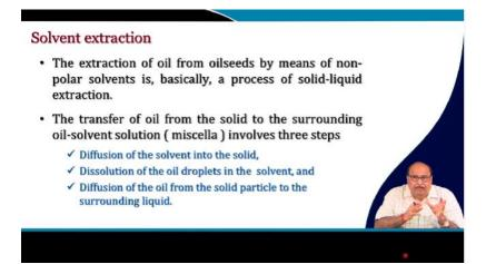
In the earlier lecture, we have seen the principle, mechanism and techniques. The extraction of oil from the oil seeds by means of a non-polar solvent and is basically a solid liquid extraction process.
