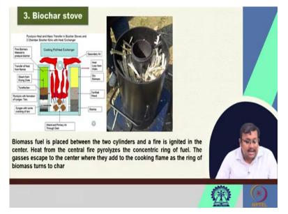
And the third method is biogas, biochar stove method. Now, this is the internal structure of the biochar stove and this is the actual biochar stove. So, in this biochar stove basically biomass fuel is placed between the 2 cylinders so you can see here there are 2 cylinder, one cylinder and second cylinder. So, the biomass material is placed between the 2 cylinders and a fire is ignited in the center. So, we pack the biomass in between the 2 cylinders and the fire is ignited in the center.
