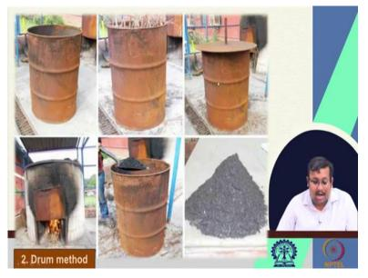
The second method is known as the drum method you can see the pictures of drum method preparation of biochar.
