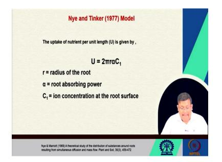
They Nye and Tinker in 1977 given a model shows you know which shows the uptake of nutrient per unit length. So this is basically given by this two pi r then alpha c one where these r stands for the radius of the root and alpha stands for the root absorbing power and c one stands for the ion concentration at the root surface.
