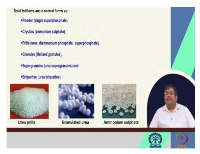
So, if we consider the solid fertilizers, solid fertilizers can be produced in several forms. For example, in the powder form, for example, single super phosphate, crystal, crystalline form like ammonium sulfate, in prills like urea, diammonium phosphate or DAP and super phosphate or single super phosphate. So, single super phosphate can be produced both in powder form or in pills form.
