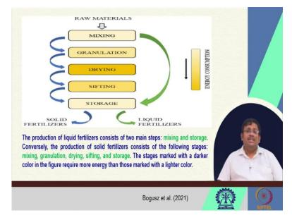
Now, the production of these solid fertilizers and liquid fertilizer can be summarized in this following flowchart. So, you can see the production of liquid fertilizer consists of 2 major steps one is mixing and that is storage. Now, conversely, the production of solid fertilizers consists of the following stages like granulation like mixing then granulation then drying, then sifting and finally, storage.
