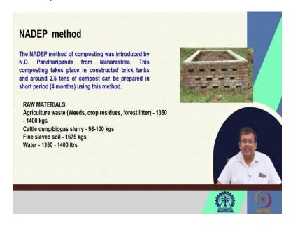
The final composting method which we are going to discuss is called NADEP method. So, this NADEP method of composting was introduced by this fellow N.D. Pandharipande from
