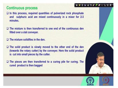
Now, let us discuss, also this is the batch process we have considered. Now we are going to discuss about the continuous process. Now, in this continuous process of single superphosphate production. It requires, required quantities of pulverized rock phosphate to react with sulfuric acid, and it is mixed continuously in a mixture for 2 to 3 minutes. Then this mixture is transferred to one end of the continuous den fitted over a slat conveyor. And, then the mixture solidifies in the den.
