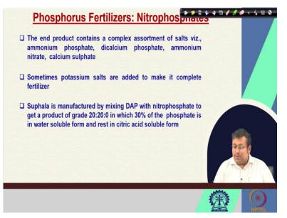
So, the end product of this nitrophosphate manufacturing process contains a complex assortment of salts, what are these? These are ammonium phosphate, dicalcium phosphate, and ammonium nitrate, calcium sulphate. So, sometimes potassium salts are also added to make it complete fertilizers.
