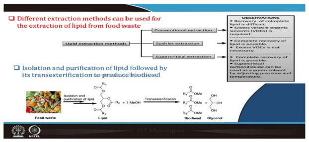
Then different extraction menthods can be used for extraction of lipid from the waste or isolation and purification of liquid followed by the transesterification to produce biodiesel. So, conventional extractions, solvent extraction and super critical extraction is being applied. So,
