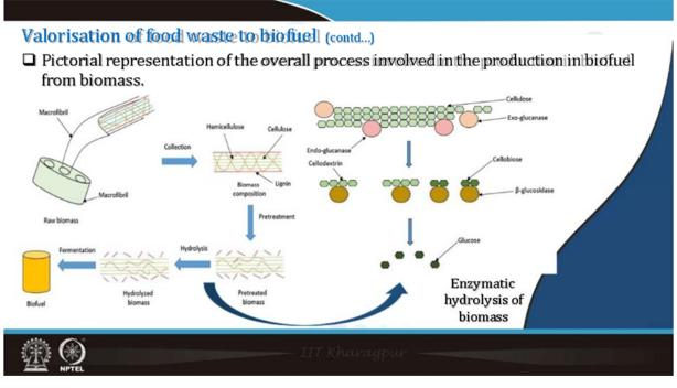
There is a pictorial representation of overall process involved in the production in biofuel from the biomass can see that you can collect a biomass that collection hemicellouse, cellouse material, then it can be given pre-treatment and hydrolysis. After that it can be fermented into bio fuel, and also hydrogen product, one can again get various product like glucose i.e by enzymatic hydrolysis, or biomass, one can also get  $\beta$ -glucosideas and cellular various products.
