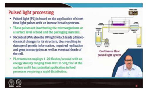
Pulsed light (PL) is based on the application of short time light pulses with an intense broad
