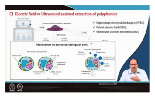
The mechanism of action basically irreversible electroporation, that is, when you are applying the electric field, then this cells are damaged, ruptured and pores are created, either existing pores are enlarged, or new pores are created. The cellular components flow to outside of cells. The solvent present in outer side penetrates into the cell and this releases polyphenolic components and cellular material. Finally, the extract component is obtained.
