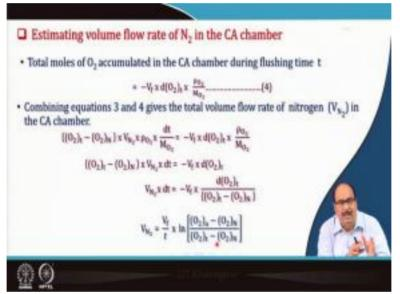
Estimate the volume flow rate of nitrogen in the CA chamber
