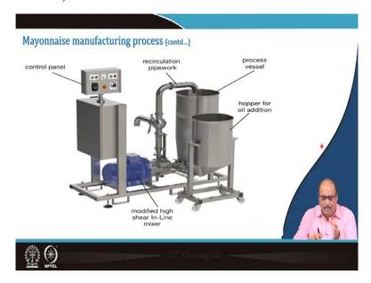
So, this is a setup machine where in these tanks various ingredients such as liquid and solid ingredients are mixed at a controlled rate. The Control panel is used for setting and controlling the parameters.
