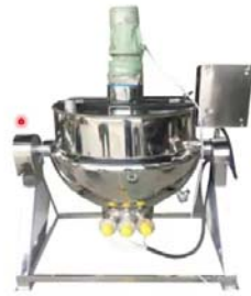
Sugar syrup is prepared in hot steam jacketed kettle
