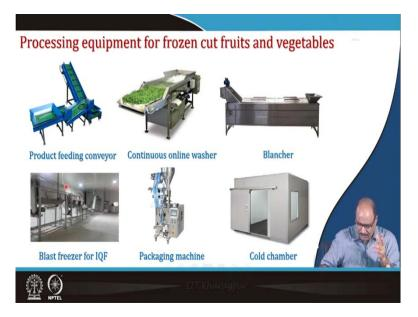
These are the equipment, possible processing equipment for frozen cut fruits and vegetables. In the continual line, these are the minimum equipment we are suggesting. They are very standard. It is being easily available like feeding conveyor, continuous on-line washing machine, then appropriate branching system.
