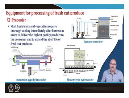
So, equipment, the operation process we studied in the earlier lecture. So, the various equipment that is the pre-cooling. So, you can say that the immersion hydrocoolers or shower type hydrocooler or vacuum pre-coolers. These are the equipment used for pre-cooling of the produce before it is sent for slicing or cutting operations.
