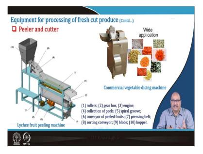
Then peelers and cutters, you can see these machines are here. That is one lychee fruit-peeling machine is shown which has various components like rollers, gearbox, engine and collections of peels. So, it is basically provided with the conveyor and also the spiral which is containing spiral grooves, so, the material comes with these hoppers comes inside the spiral groove and basically by this rubbing action the peels are removed.
