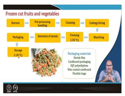
Then frozen cut fruits and vegetables, the process technology include the harvesting after that preprocessing and handling, cleaning, cutting, slicing, blanching, the freezing, detection of metal, packaging and storage at minus 18 degree Celsius. There is freezing operations, at low temperature, all the water present in the material in the fresh cut produce is frozen and converted into ice and then this frozen is appropriately packed and after that it is stored at minus 18 or minus 23°C.
