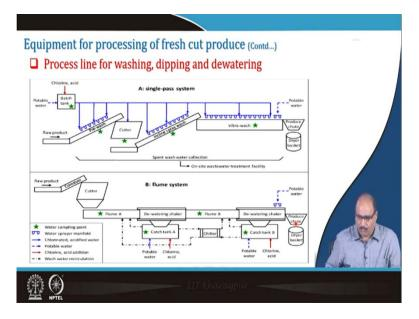
This is the process line for washing, dipping and dewatering of fresh cut fruits and vegetables, may be a single pass line. Here you can see that the raw produce comes and it is a portable water which containing some appropriate amount of chlorine or acid etc. So, it is sprinkled here and the commodity is washed. And after that it is sent for the cutting operation and cut vegetables. It is a basic conveyor. It is inclined spray wash.
