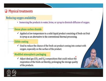
So, reducing the oxygen availability, physical treatment may be immersing the product in water, brine, syrup to diminish diffusion of oxygen, dense phase carbon dioxide, applied low
