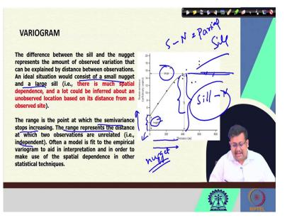
So, in the Variogram there are different types of parameters, you should understand that here we are putting the distance and here we are putting the semi variance. Now, you can see here the difference between the sill and the nugget represents the amount of observed variation. So, here you can see at distance 0 there is some variability, which we cannot explain in terms of distance between the points.
