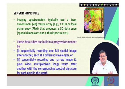
Now, if we see the sensor principal the imaging spectrometers typically uses a twodimensional 2D matrix array, a CCD array or focal plane array that produces the 3D data cube, we already know that in case of hyperspectral remote sensing we need to have a 3D data cube. So, the output is a 3D data cube.
