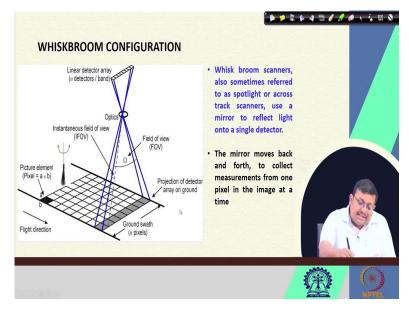
So, let us discuss, how we can generate these hyperspectral data cube? There are two types of scanner, while we talk about the hyperspectral imager, there are two types of scanner. One is whisk broom scanner another is a push broom scanner. Now, this whisk broom scanner, we can see this is a whisk broom configuration.
