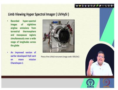
And, then come the LiVHySI the LiVHySI is the short form of Limb Viewing Hyper Spectral Imager and it was an improved version of earlier developed HySI sent in moon mission Chandrayan- 1. So, and this this LiVHySI basically recorded the hyperspectral images of nighttime airglow emissions from terrestrial thermosphere and mesopause region simultaneously over a wide range of longitude across the globe.
