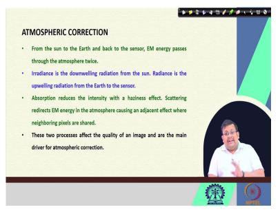
And, what is atmospheric correction? Atmospheric correction that from sun to the Earth and back to the sensor, these electromagnetic energy passes through atmosphere to twice. One during the incoming radiation and there is outgoing radiation. Now, irradiance is the down welling radiation from the sun, whereas, radiance is the upwelling radiation from the Earth to sensor.
