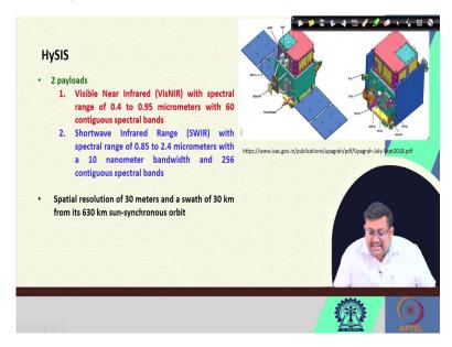
So, in this HySIS, there are two payloads. So, these two payloads are basically first one is the visible near Infrared with spectral range from 0.5, 0.4 to 0.95 micron with 60 contiguous spectral band this is the first payload, the second payload was shortwave Infrared range with spectral range of 0.85 to 2.4 micron with a 10 nanometer bandwidth and 256 contiguous spectral bands.
