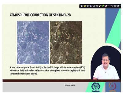
So, here you can clearly, clearly see that an example of atmospheric correction of SENTINEL-2B, of course, this is a multispectral sensor, but you can have an idea. So, here it is a true color composite of SENTINEL-2B image with top of the atmosphere. So, this is the top of the atmosphere reflectance and this is the surface reflectance after atmospheric correction with the land surface reflectance code.
