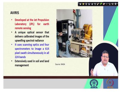
So, these AVIRIS has been lately utilized extensively for different types of agricultural purposes and land use management. So, these AVIRIS was first developed, it was actually developed in Jet Propulsion Laboratory for Earth remote sensing and this is a unique optical sensor that delivers calibrated images of the upwelling spectral radiance, it uses scanning optics and four spectrometers to image a 614 pixels worth simultaneously in all 224 bands.
