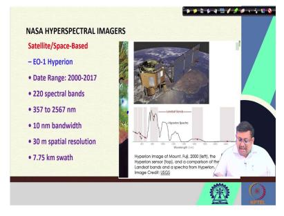
So, let us see the features of EO-1 Hyperion as I have told you that this sensor has been already decommissioned. So, these EO-1 Hyperion the date, the date range for which the data is available is from 2000 to 2017. And it has 220 spectral bands, which ranges between 357 to 2567 nanometer and it has 10 nanometer bandwidth with 30 meter spatial resolution with the 7.75 kilometers swath.
