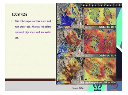
Blue color, as you can see here also in this picture, you can see there are two images one was taken at 2019 and other is 2020. And you can see the percentage changes from 2019 to 2020. And so, evaporative stress, how it changes from 19 to 20 we can clearly see so in this image is blue color represents the low stress and high water use whereas the red color represents the high stress and low water use. So this is the application of ECOSTRESS.
