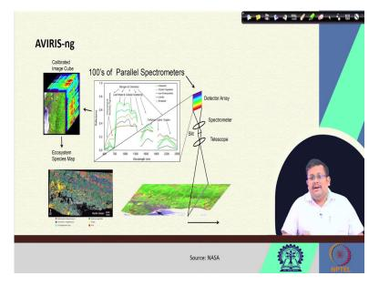
Now, you can see a simplified flowchart, how these AVIRIS-NG generally works. So, it has spectrometer which captured the images and ultimately it produces the calibrated image cube for producing the ecosystem species map, for example. So, these AVIRIS-NG has been lately utilized in different countries for producing or for capturing the high level details from the Earth features.
