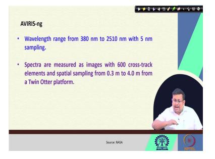
So, these wavelength range for these AVIRIS-NG generally ranges from 380 to 2510 nanometer with 5 nanometer sampling and spectra are measured as images with 600 cross-track elements and spatial sampling from 0.3 to 4 meter from a Twin Otter platform. So, this AVIRIS-NG has been flown to different areas from over the water body, over the land surface over the crop fields, over the different types of mountains and glaciers to capture their images and subsequent analyze them.
