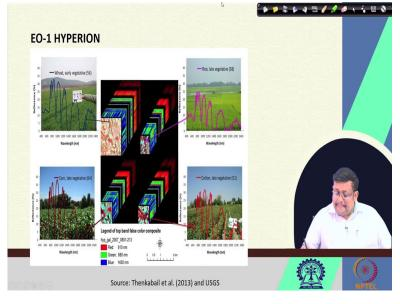
Now, these are also the hyperspectral spectra obtained from Hyperion for a given pixel. So, as we know that in case of hyperspectral remote sensing we get a data cube which is bounded by X and Y direction and in the Z direction we get the wavelengths.
