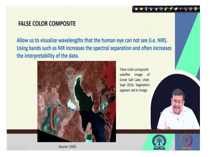
Now, if we go to the next slide and we will see that false color composite. Now, the false color composite allows us to visualize the wavelengths that human eye cannot see, of course, in the near infrared range, in the near infrared rays we cannot see by our naked eyes. So, we need some false color composite we need some color to indicate the features from the near infrared image images.
