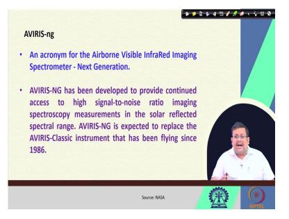
Now, AVIRIS-NG, now AVIRIS-NG, what is AVIRIS-NG. AVIRIS-NG is an acronym for the Airborne Visible InfraRed Imaging Spectrometer - Next Generation. So these AVIRIS-NG has been developed to provide the continued access to high signal to noise ratio imaging spectroscopy measurement in the solar deflected spectral range, and it is expected to replace the average classic instrument that has been flying since 1986.
