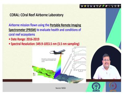
Now, another one is called the PRISM. So, PRISM stands for Portable Remote Imaging Spectrometer which is, which is there in the Coral Reef Airborne Laboratory or Coral to evaluate the health and conditions of coral reef ecosystem, it date range from 2016 to 2019 and the spectral resolution varies from 349.9 to 1053.5 nanometer with the 3.5 nanometers sampling.
