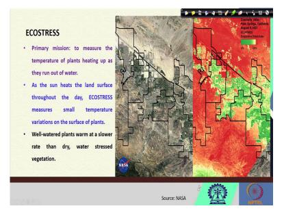
And, what is the, what is the mission of ECOSTRESS? So, mission of ECOSTRESS is to measure the temperature of the plants heating up as they run out of water. So, evaporative stress measurement is the major mission for ECOSTRESS sensor. Now, as the sun heats the land surface throughout the day, ECOSTRESS measures the small temperature variation on the surface of the plants. And remember that of course well water plants warm at a slower rate than dry, water stressed vegetation.
