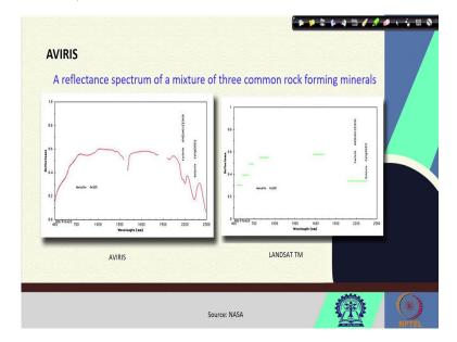
So, you can clearly see these AVIRIS reflectance spectrum of a mixture of three common rock forming mineral. Here you can see that so, this is the AVIRIS spectra and the same spectra which were taken by multispectral lens or thematic map and so, you can clearly see the difference of the information difference in information we can gather from evidence as compared to any other multispectral sensor.
