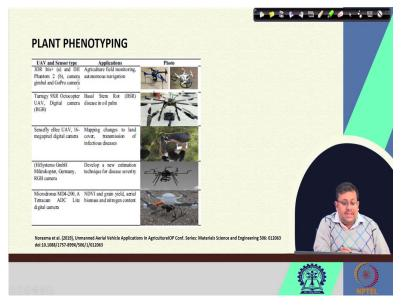
So, let us see some examples of UAV. One of the major example of UAV is plant phenotyping. So, for example some examples are given here. If you consider these 3DR Iris4, and then DJI Phantom 2, with a camera gimbal and GoPro camera. So, these type of UAV and sensor combinations are useful for agriculture film monitoring and autonomous navigation. So, some the photographs are given here.
