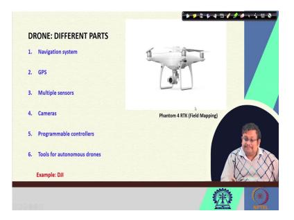
So, what are the different parts of a drone? As you can see, here this is an example of a agricultural drone Phantom 4 RTK, which is being used for field mapping. And these drones have different types of parts like navigation system, it has global positioning system, or GPS, it has different multiple sensors, they have cameras, programmable cameras, as well as tool for autonomous drones are also there.
