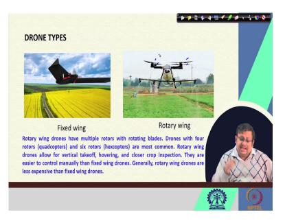
There are two broadly there are two types of drones one is called the fixed wing drones another one is the rotary drone. So, fixed wing drones are having the fixed wings and their advantage is they can cover a large area of the field within a very short period of time because of their fixed wing operations. Another type of drone is called the rotary drone, and it is the mostly, the majority of the agricultural drones are rotary drones.
