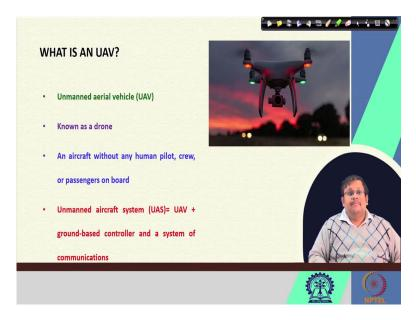
So, the first question comes to our mind, what is an UAV? Now UAV is the short form of Unmanned Aerial Vehicle, and of course, that is also known as a drone, which is basically an aircraft without any human pilot, crew or passengers on board. So, there is another term called UAS or Unmanned Aircraft System. So, this UAS is basically a combination of UAV plus ground based controller and a system of communications.
