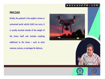
So, if we see, what is a payload? Payload is the weight of the drone, the weight a drone or unmanned aerial vehicle can carry. So, it is usually counted outside the weight of the drone itself, and it can include anything additional to the drone, such as extra cameras, sensors or packages for delivery.
