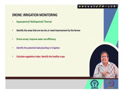
Now, what are the importance, what are the other application of NIR drone? So, for agriculture as you can see here we can use this drone for irrigation monitoring using either hyperspectral or multispectral or thermal sensor data, we can identify the areas that are too dry or needed improvement by the farmers, and using this drone survey, it is possible to improve the water use efficiency, and you can already, using this drone you can identify or recognize the leaks or pooling of in irrigation.
