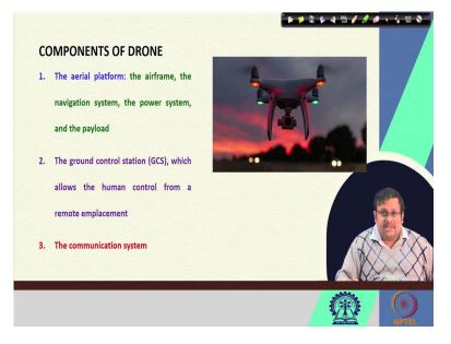
Now, what are the major components of the drone? So, in a broad sense, a drone can be composed of three major part. One is the aerial platform, second is the ground control system, and the third one is the communication system. So, the aerial platform basically composed of airframe, the navigation system and the power system, and the payload. So, these are very, very important terminologies, the airframe, the navigation system and the payload.
