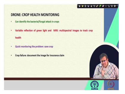
Also these drone can be used for crop health monitoring, because using this drone survey you can identify the patches which are showing the bacterial or fungal attack of the crops, you can also get the variable reflection of the green light and NIRS, and then you can, and also using that multispectral images, can track the crop health by using the reflection of the green and NIRS.
