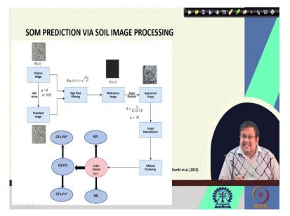
Our group has also did some research for using the smartphone captured image from the same setup and in combination with some image processing. So, you can see that, after we took the image we did some image processing like we pass the image through high pass filtering. I will tell you what is high pass filtering. So, when the image was passed to the high pass filters, we retain only the reflectance image and we removed the intensity values from the image.
