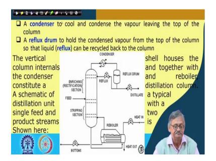
A condenser to cool and condense a condenser to cool and condense the vapour leaving the top of the column. A reflux drum right reflux means some product which has come and again being fed that is called reflux. So, a reflux drum to hold the condensed vapour from the top of the column so that liquid reflux can be recycled back to the column right.
