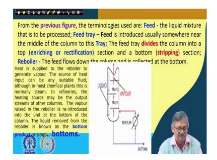
So, then we come to this from the earlier figure which we have just shown the terminologies which you are used are like this feed that is the liquid mixture that is to be processed it is mixture of the separating liquids. Feed tray through which feed is introduced usually somewhere near the middle of the column right which we have shown just it was at the somewhere middle of the column; it was the column, it was the feed somewhere middle right.
