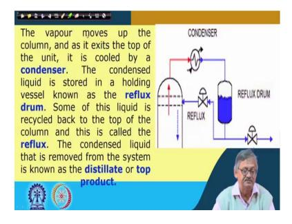
The vapour moves up if we look at even in the previous one also here also that the liquid is this right coming down and the vapour through this reboiler is going through this up right. So, liquid with the blue color it is coming down and the vapour is going up. So, like that it is coming to the reboiler, from the reboiler vapours are coming and then going through the column this is how it is.
