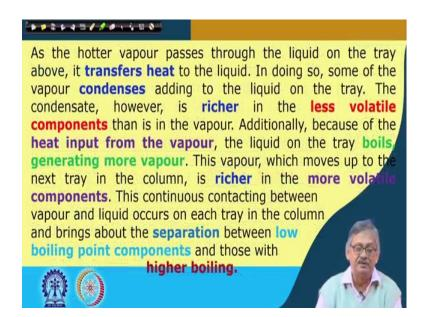
As the hotter vapour passes through the liquid on the tray above, it transfers heat to the liquid, so, there is a vapour and liquid heat exchange. In doing so, some of the vapour condenses adding to the liquid; so, while it was going so, this was the vapour, this was the liquid. So, some liquid and vapour got the exchanged and a little vapour got condensed it came out and a little liquid way we came vapour it went up like that right. So, condenses adding to the liquid on the tray.
