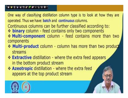
One way of classifying distillation this is done by columns right. So, number of things are there so, we will also look into in detail that. So, that is why it is called column. So, one of the classifying way of classification of distillation column type is to look into at how they are operated. So, we have batch type, as I said there steam distillation and continuous columns both.
