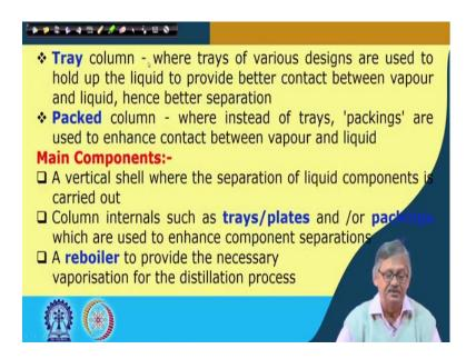
Tray: tray column is where the trays of various designs are used to hold up the liquid to provide better contact between vapour and liquid, hence better separation etcetera. Packed columns – where instead of trays, packings are used to enhance contact between vapour and liquid. The main components of the column are a vertical shell where the separation of liquid components is carried out.
