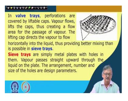
In valve trays, that was for bubble cap, this was for bubble cap these are bubble cap and this is called bubble cap arrangement in the tray. For valve trays per perforations are covered by liftable caps, which can be physically lifted. Vapour flows, lifts the caps, thus creating a flow area for the passage of the vapour. The lifting cap directs the vapour to flow horizontally into the liquid, thus providing better mixing than is possible in sieve trays.
