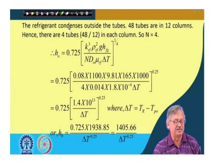
If this  $h_i$  is known, then the refrigerant condenses outside the tubes right. The refrigerant condenses outside the tubes 48 tubes are in 12 columns. Hence there are 4 tubes 48 over 12 in each column. So, N is equal to 4; 48 tubes 12 columns, so we have 48 by 12, there is 4 number of tubes in each column, right.
