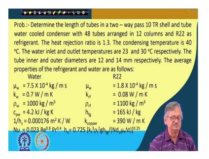
And in that case the problem which was given is like this; that determine the length of tubes in a two way pass 10 ton refrigeration TR, right. This TR is generally in refrigeration used and that is called tonnage of refrigeration, 10 ton refrigeration TR or 10 TR it is in short said, shell and tube water cooled condenser.
