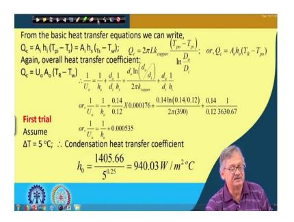
From the basic heat transfer equations we can write that what  $Q_c = A_i h_i (T_{pi} - T_s) = A_i h_s$ ( $T_s - T_w$ ); where and  $Q_c$  that can be written as  $2 \pi L k_{copper} (T_{po} - T_{pi})$  right divided by ln ( $D_o / D_i$ ); or  $Q_c = A_o h_o (T_r - T_{pa})$  right. Again overall heat transfer coefficient that can be written as;  $Q_c = U_o A_o$  or  $U_o A_o (T_r - T_w)$ .
