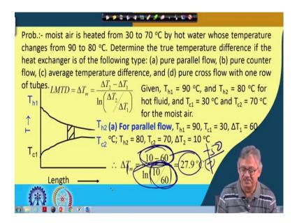
Then  $\Delta T_{mean}$  or log mean we can write is 10 that  $T_2 \Delta T_2 - \Delta T_1$ . So, 10 - 60, 'right'. Let us erase.  $(10 - 60) / \ln (10 / 60)$ , 'right'. So, (10 - 60) is -50 and if you take 10 / 60 that is 1 / 6 ln (1/6) that will have some value with negative.
