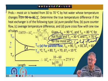
It is like this that, moist air is heated from 30 °C to 70 °C by hot water whose temperature changes from 90 to 80 °C. Determine the true temperature difference if the heat exchanger is of the following type. Number 1, pure parallel flow, number 2, pure counter flow, number 3, average temperature difference and number 4 pure cross flow with one row of tubes. So, there is no multiples, nothing, nothing single, 'right'.
