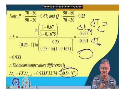
So, out of this 4 we see that  $\Delta T$  counter current, 'right', that gave a value which is very very good, but that was very close to the average,  $\Delta T$  average. Since, the temperature differences were small, so  $\Delta T_{lm}$  values were not that significantly different. But if the  $\Delta T_m$  is or rather if the difference of temperatures are very high then definitely the on the  $\Delta T_{lm}$  or LMTD that will be highly appreciated.
