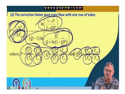
Then it is remaining that is 4th. Fourth one was that what is the temperature for LMTD. For the cross flow cross now for flow we have  $F = \Delta T_{lm}$  or mean over  $\Delta T_m$  cross flow or mean temperature log mean temperature for cross flow that is the F.
