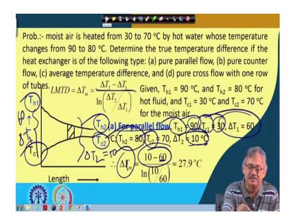
So, if this is true, then we can write for parallel flow  $T_{h1} = 90^{\circ}$ ,  $T_{c1} = 30^{\circ}$ , so  $\Delta T_1 = 60^{\circ}$ . So,  $T_{h1} = 90^{\circ}$ ,  $T_{c1} = 30^{\circ}$ , so this is the  $\Delta T_1$ , 'right'. And  $T_{h2}$  is 80°, so this one is 80° and  $T_{c2} = 70^{\circ}$ , so this one is 72°. So, their difference is  $\Delta T_2 = 10^{\circ}$ C. So, that  $\Delta T_1$  came to be 60 and this  $\Delta T_2$  came to be 10°.
