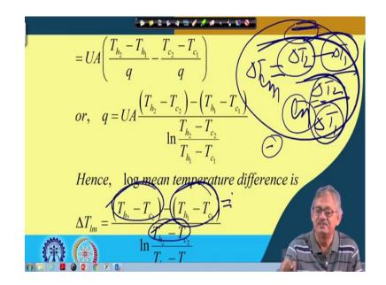
Now, this can be simplified and written as T, that  $\Delta T_{lm}$  or let us write here  $\Delta T_{lm}$  is equal to this we can write  $\Delta T_2$  and this we can write  $\Delta T_1$  over 1n of this we can write  $\Delta T_2$  and this we can write  $\Delta T_1$ .
