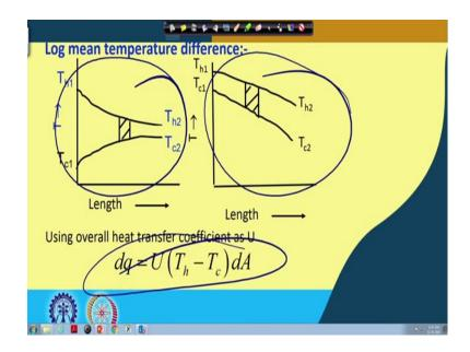
So, let us quickly look at where we were that is we started here that log mean temperature difference I am not going to emphasize again on this. This was for counter current and this was for co-current and this is the general equation; general equation for heat transfer, 'right'.
