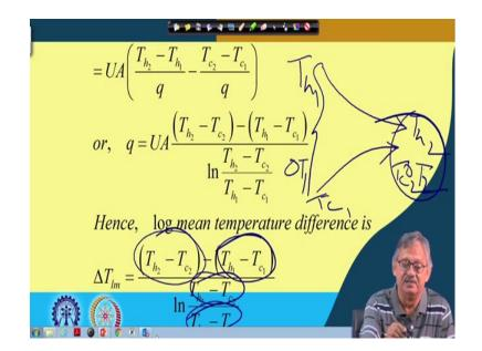
Let us look into really this is one, this is another, 'right', so  $T_{h1}$  and this is  $T_{h2}$  and this is  $T_{c2}$  and this is  $T_{c1}$ , 'right'. And this  $T_{h1}$  -  $T_{c1}$  is this one and  $T_{h2}$  -  $T_{c2}$  is this one, 'right'. So, this is what? Say we say  $\Delta T_2$  and say this is  $\Delta T_1 \ln (\Delta T)$  it is 2 -  $T_{c2} / T_c$ ,  $T_{h1}$  -  $T_{c1}$ .
