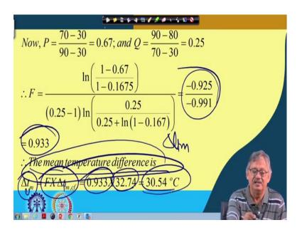
So, with all this parameters let us substitute the values and we get that P = (70 - 30)/(90 - 30) that is 0.67. Q = (90 - 80) / (70 - 30) that is 0.25. And then  $F = \ln ((1 - 0.67)/(1 - 0.1675)) / (0.25 - 0.1) \times \ln (0.25 / (0.25 + \ln(1 - 0.167)))$  which comes on simplification as minus on the numerator -0.925 and on the denominator -0.991. So, this ratio comes to be 0.933, 'right'.
