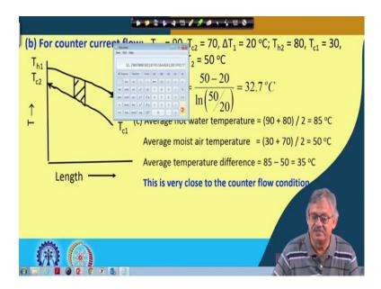
So, we got 32.7 as the  $\Delta T$  log mean for counter current, 'right'. So, for counter count we got 32.7 °C as the log mean temperature difference, 'right'. Now, third one was available temperature. So, average temperature of the hot fluid is what? So, this was  $T_{h1}$  and this was  $T_{h2}$ . So,  $T_{h1}$  was 90 and  $T_{h2}$  was 80. So, average of that is 85 °C. So, average temperature of the inlet or fluid is 85 °C.
