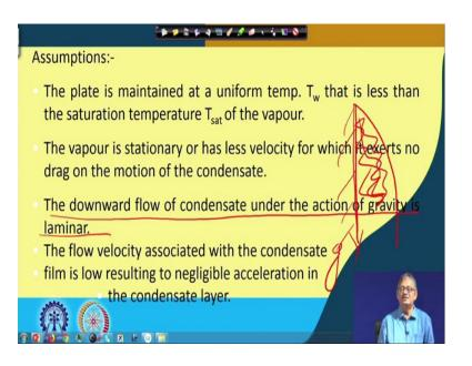
So, if this is known, then we can do the analysis like this with certain assumptions, and assumptions are valid assumptions like this. That the plate is maintained at uniform temperature  $T_w$  wall temperature that is less than the saturation temperature  $T_{sat}$  of the vapor. This is first assumption that is the plate is maintained at a temperature  $T_w$  which is less than the saturation temperature of the vapour or  $T_{sat}$ , 'right'.
