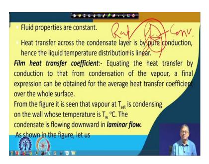
So, only conduction through the fluid, there is no convection or radiation it in this, 'right', so that is another very basic assumption.
