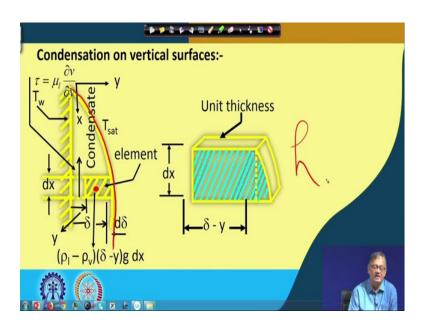
So, we know that this flow we will find out what is the temperature distribution, what is the heat transfer coefficient, etcetera we will find out. So, to do that, we keep this thing in mind that our volume element is this having  $(\delta - y)$  in the y direction, in x direction dx and the third dimension is unity or unit thickness, 'right'.
