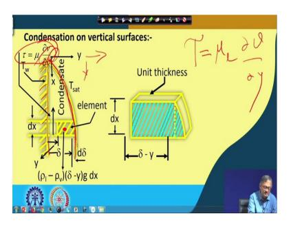
So, let us look into that how first we take picture that this is drawn with me of course that we are taking that the one which we said a vertical wall, 'right'. So, this is the vertical wall and there is a flow of the fluid, and the flow is like a parabolic flow, 'right' that in pipe flow also you have seen that flow can be parabolic, 'right'.
