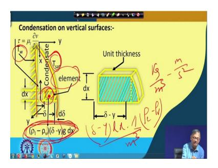
So, this is the volume element; volume is your  $(\delta - y) \times dx \times 1$  that is the volume, 'right', and  $(\rho_1 - \rho_v)$  is the density difference that is in this, this is m<sup>3</sup> and that is kg/m<sup>3</sup>, 'right', and g is m/s<sup>2</sup>, 'right'. So, we get kg/m<sup>3</sup> that m/s<sup>2</sup>; this unit we will utilize a while and that is applicable at this point, 'right'.
