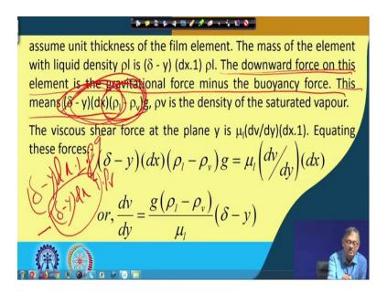
So, because the gravitational force is that volume  $(\delta - y) \times dx \times 1$  that times  $\rho_1 \times g$  that is the gravitational and minus that for the vapour it was equivalent  $(\delta - y) \times dx \times 1 \times \rho_v$ , 'right'. So, we take  $(\delta - y) \times dx \times 1$  as common, then we get  $\rho_1 \times \rho_v$  and g common so that comes to  $(\delta - y) \times dx \times (\rho_1 - \rho_v) \times g$ , where  $\rho_v$  is the density of this saturated vapour.
