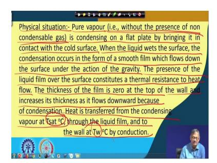
So, as we said just now that physical situation if we elaborate that the physical situation is like that. We have a pure vapour that is without the presence of non condensable gas, 'right', we have pure vapour without the presence of non-condensable gas is condensing on a flat plate by bringing it in contact with cold surface. When the liquid wets the surface, the condensation occurs in the form of a smooth film which flows down the surface under the action of gravity.
