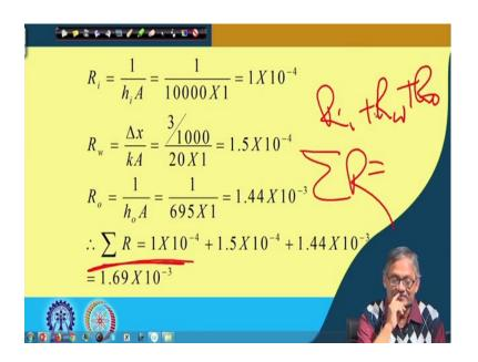
So,  $R_i$  is  $1/h_iA$ ,  $R_i$  is  $1/h_iA$  that is  $1/(1000 \times 1)$ , 'right',  $h_i$  has been given 1000; 10000. So,  $1/(1000 \times 1)$ ; that means,  $1 \times 1 \times 10^{-4}$  that is  $R_i$ , 'right'. What are these  $R_i$ ?  $R_i$  is if you remember we had this and then we had this, then we had a jacket inside which that steam is condensing, 'right'. So, we have one resistance here with h i, 'right' that we have found out  $R_i$ . So, this is the film resistance or the wall.
