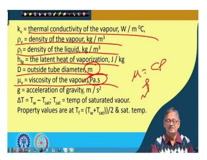
So, that is what is  $k_v$  is the thermal conductivity of the vapor in W/m°C,  $\rho_v$  is the density of the vapor in kg/m<sup>3</sup>,  $\rho_l$  is the density of the liquid in kg per meter cube,  $h_f$  g is the latent heat of vaporization in J/kg, D is the outside diameter of the tube in meter, a  $\mu_v$  is the viscosity of the vapor in Pascal seconds, this is in Pascal seconds mind it.
