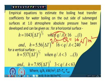
However, here we are using q/A that is Q and this is 16, not q this is q/A that is flux W/ m<sup>2</sup> ok. So, that empirical relation is in the horizontal surface. It is 1043  $\Delta T^{1/3}$  when it is < 16 and h is 5.56  $\Delta T^3$  where q/A is between 16 and 240. For vertical surfaces h is 537  $\Delta T^{1/7}$  when q/A < 3, whereas, h is 7.95  $\Delta T^3$ , when q/A is between 3 and 63, 'right'.
