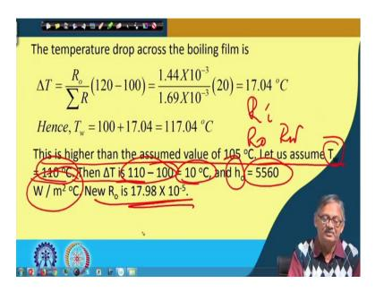
Now, reassumption will be there, 105, let us assume that 110 °C is the wall temperature, 'right'. Then delta T is 110 - 100 or 10 °C, 'right' and h<sub>o</sub> why that equation we got 5560, 'right', 5560 W/m<sup>2</sup> the same equation which we have used 105 °C. And by the same way you found out R<sub>i</sub>, R<sub>o</sub> and R<sub>w</sub>, 'right'. So, you can find out all of them. And new R<sub>o</sub> is now  $17.98 \times 10^{-5}$  by the same process we have found out, 'right'.
