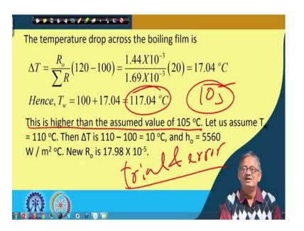
Now, if we find out again q, q becomes the temperature drop actress the boiling film is  $\Delta T$  is equal to  $(R_0/\Delta R) \times \Delta T$  that is (120 - 100). So,  $R_0$  is  $1.44 \times 10^{-3}$ , summation of R is  $1.69 \times 10^{-3}$  and this  $\Delta T$  is 20, so 17.04. So, the wall temperature becomes 100 +17.04 is 117.04 which is much above the assumed which was 105, 'right'. So, this is higher than that assumed value of 105 °C. So, first assumption it did not leak.
