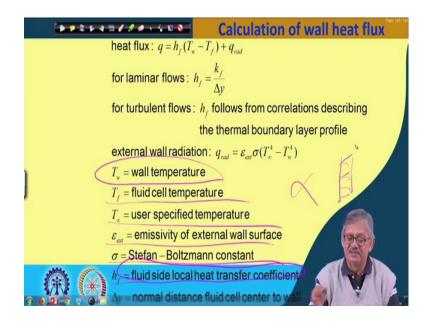
So, if this is known then let us go for calculation of wall heat flux. So, if we want to find out the wall heat flux, then heat flux q is  $h_f \times (T_w - T_f) + q_{radiation}$  and for laminar flows  $h_f$  is  $k_f/\Delta y$ , for turbulent flows  $h_f$  follows from correlations describing the thermal boundary layer profile.
