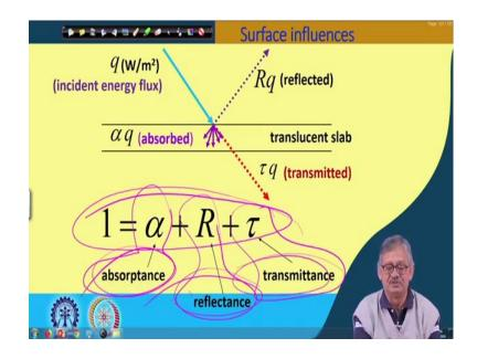
However, we must do some basics and show that when a radiation is coming that is incident energy flux like this, 'right", q W/m<sup>2</sup> that is the incident energy flux, and this is the surface which is a translucent slab. So, out of this when it is incident, then  $\alpha q$  quantity is absorbed, Rq quantity is reflected, and  $\tau q$  quantity is transmitted, 'right".
