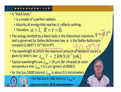
The wavelength at which the maximum amount of radiation occurs is given by another law which is called Wien's law, 'right"; which is called Wien's law. And this is  $\lambda_{max}T = 2.898 \times 10^{-3}$  m.K, 'right",  $\lambda_{max}$  is meter T is in Kelvin. So,  $\lambda_{max}$  T is 2.898, 10<sup>-3</sup> m.K.
