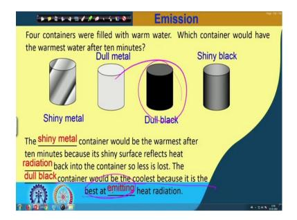
Now, we have said earlier one term that epsilon or emissivity, 'right". So, that emissivity or emission how can we measure or to have some idea, let us look into this. Those 4 containers were filled with warm water, which container would have the warmest water after 10 min? One, shiny metal container with shiny metal, container made of dull metal, container made of dull black and container made of shiny black.
