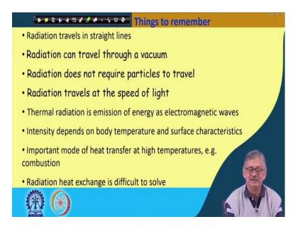
So, for this the certain things are to remember for radiation heat transfer, that radiation travels in straight lines. Radiation can travel through a vacuum also because the space is that where there is nothing no medium, but still it is propagating. Radiation does not require particles to travel. Radiation travels at the speed of light. Thermal radiation is emission of energy as electromagnetic waves. Intensity depends on body temperature and surface characteristics.
