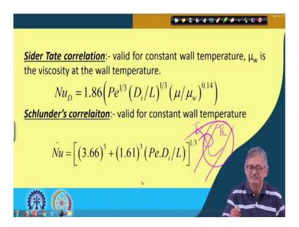
So, when we had this flow. So, the viscosity at the wall which was  $T_{\infty}$  around and viscosity at the center which is say  $T_i$  around, 'right' are quite different. So, unless you take care of this viscosity correction then you will have some error. So, that is what the Sider Tate correlation has incorporated that.
