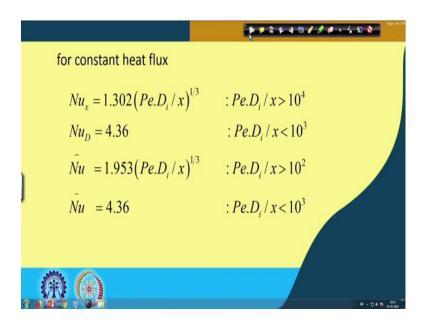
So, if this is true then for constant heat flux, again under different conditions for constant heat flux  $Nu_x = 1.302(Pe.D_i/x)^{1/3}$ , where  $Pe.D_i/x > 10^4$ . Whereas, Nu<sub>D</sub> is means Nusselt number in terms of diameter is 4.36. This is also valid for P<sub>i</sub> into D<sub>i</sub> sorry  $Pe.D_i/x < 10^3$ . Average Nusselt number is  $1.953(Pe.D_i/x)^{1/3}$  that is  $Pe.D_i/x > 10^2$ .
