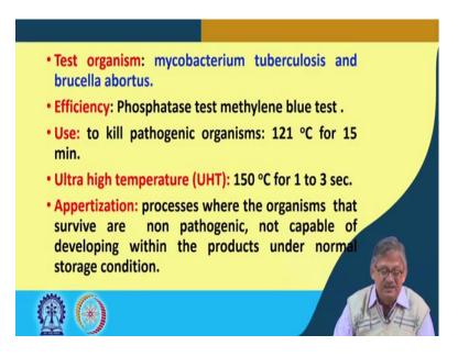
So, you can see afterwards. Test organism is mycobacterium tuberculosis and brucella abortus, 'right'. Efficiency is determined by phosphatase test methylene blue test this way 'right'. It is used to kill the pathogenic organisms 121 degree centigrade for 15 minute and Ultra high temperature around 150 degree centigrade for 1 minute or 1 to 3 second so, that is used.
