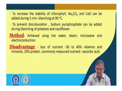
Other reasons for doing the doing the blanching is to increase the stability of the chlorophyll, sometimes sodium carbonate and calcium oxide is used and during the 3 minute blanching at 90 degree centigrade in many cases and also it prevents the discolouration.
