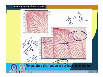
T at any place t at any place minus  $T_{\alpha}/T_i - T_{\infty}$ , 'right'. So, this is for the long cylinder, 'right' and here also if we know Fourier number there is alpha T by instead of L it is L for slab it is  $r_o$  square, 'right', that if we know r value of r then you know the value of Fourier number, then from that Fourier number here also you have inverse of Biot number there is 1/Bi that is hL/k. So, k/hL that value if you know, then you can point that where it is on the graph.
