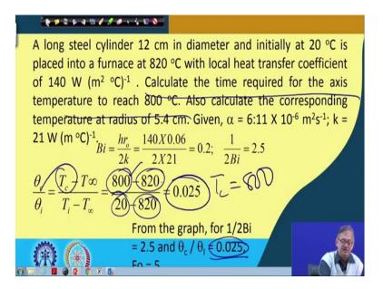
So, 0.025 we have found out and from there we have this centre temperature we can find out there is from the graph of this, this is 0.025, 'right' and this why we have made 800 minus 820 this is the environmental temperature, initial temperature, environmental temperature, 'right'. So, here we should first find out because 800 degree centigrade we have not shown.
