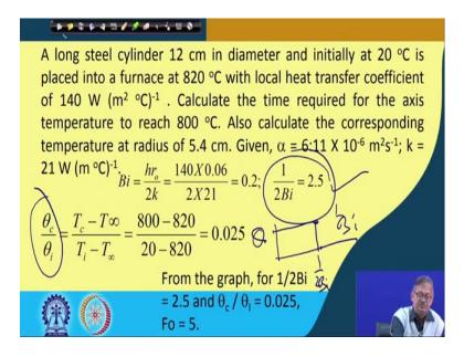
So, we have found out what is the value of 1 by 2 Bi which is 2.5. So, we have found out this; so, theta c by theta i. Now again we go to that plot where we have to find out 1/2Bi, 'right'; so, 1/2Bi versus  $r_o/ri$  so, that here it is centre temperature. So, centre temperature is 1 by Bi so, from there we get this value and get the value of theta, 'right'. So, the  $\theta_c / \theta_1$  that has come to be 0.025, 'right'.
