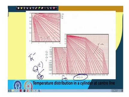
So, this is the Heisler chart for long cylinders, 'right' where  $\alpha t/L_{r0}^2$  square instead of L
