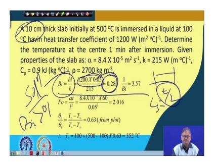
So, for the solution what do you need? First you look into that what is the value of Bi. So, Bi is hl/k; this is for slab. So, it is given 10 centimetre. So, 10 centimetre is the thickness. So, t/2 is the characteristic Length; so, L<sub>s</sub> being t/2. So, it is 10 centimetre
