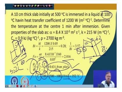
Then again what we need to do? We need to go to that theta versus Fourier number that plot, 'right' which was like this for different 1 by Bi. So, for a given Fourier number that is 2.06 for a given 3.57 that is this. So, we look at the point and then find out the value of
