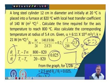
Since time was not given so, we have found out theta c over theta i and that has become 0.025,  $F_o$  is not given. So, from this value and from 1/2 this value we find out  $F_o$  value. So,  $F_o$  value came out to be 5, 'right';  $F_o$  value Fourier number came out to be 5. So, if it
