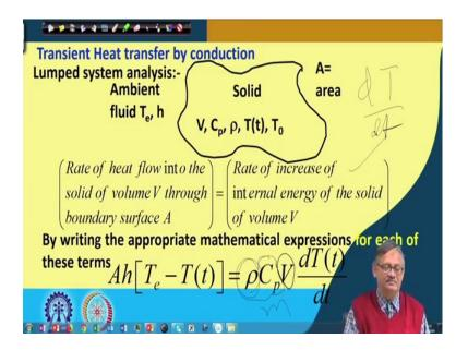
And this internal energy we have calculated as  $mC_p\Delta T$ , where m corresponded to  $\rho$  times V and this is m and  $C_p$  and  $\Delta T$  and this  $\Delta T$  is a function of time. So, that is why it is dT/dt that is rate of change of temperature with respect to time, 'right'.
