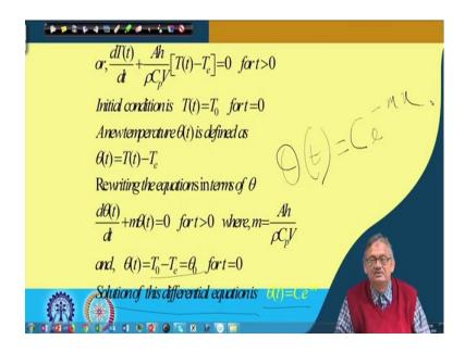
And solution of this differential equation gives in the form  $\theta_t$ , 'right',  $\theta_t$  is equal to  $Ce^{-mx}$
