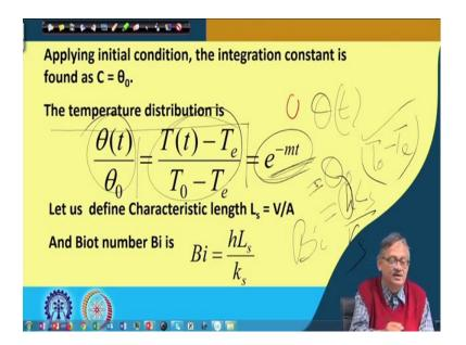
So, if that be true then the temperature distribution is  $\frac{\theta(t)}{\theta_0} = \frac{T(t) - T_e}{T_0 - T_e} = e^{-mt}$
