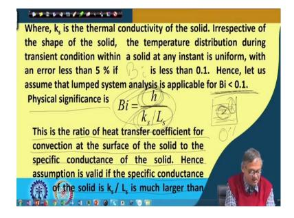
Now, where  $k_s$  is the thermal conductivity of the solid irrespective of the shape of the solid the temperature distribution during transient condition within a solid at any instant is uniform with an error less than 5 percent; if less than 0.1, 'right'; here it
