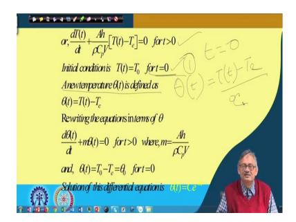
Not at time t is equal to 0 because time t is equal to 0 is the initial condition. So, this is valid for time t greater than 0. And initial condition is like this that T at any time t is equal to  $T_0$  for t is greater is equal to 0, 'right' this is the initial condition, 'right' and new temperature definition we let us define  $\theta_t$ , 'right'  $\theta_t$  let us define as a new temperature and that is to be defined as  $T_t$ - $T_e$ , 'right'.
