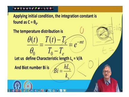
This is the very fundamental that the Biot number has to be very high which in other word is saying that is take again I gave the same example that we had bath of water under boiling condition, 'right', and we had put spherical ball in it this environmental temperature was equal to 100 degree centigrade and this initial temperature was say 25 degree centigrade.
