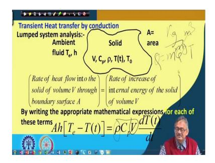
So, Q is equal to  $mC_p\Delta T$  that we know. So, to have the m we are making  $\rho$  times V, 'right';  $\rho$  is in kg per meter cube and V is in meter cube, so, it is kg-m, 'right'.
