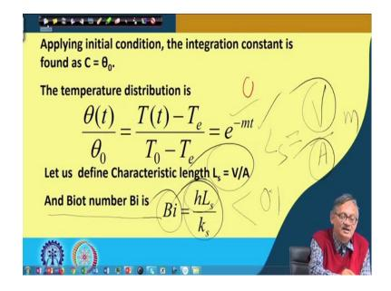
So, if this be true this is dependent on here this is valid only if that a number Biot number Bi is equal to  $Bi = \frac{hL_s}{k_s}$  here h is the transfer coefficient of the environment;  $L_s$  is the characteristic length and this is defined as equal to V over A, where V is the volume of the body, A is the surface area. So,  $L_s$  is V over A and that is in meter, 'right'. So, this is called characteristics length or  $L_s$ .
