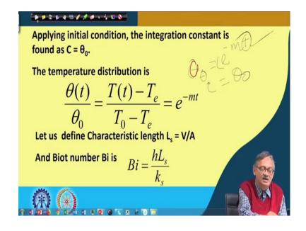
So, if it is mt then at time t is equal to 0, we can write that theta 0 theta 0 is equal to or theta t was now theta 0 and that is equal to that e to the power minus mt. So, c became equal to  $\theta_0$ , 'right' because time t is equal to 0 and is  $\theta_0$ . So, C became equal to it was Ce<sup>-mt</sup>. So, time t is equal to 0. So, it became t theta 0 and C became equal to  $\theta_0$ , 'right'.
