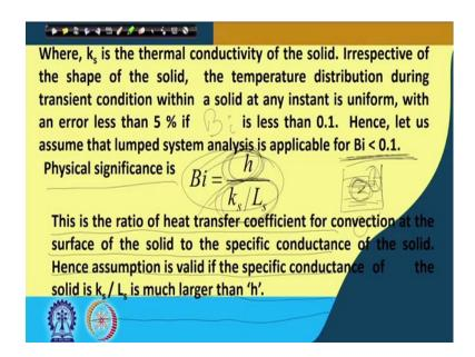
So, with this let us say that we have initiated the unsteady state heat transfer and we have seen Biot number is h over  $k_s/L_s$  and the value of it has to be less than 0.1, then only we can make the lumped system analysis, 'right'.
