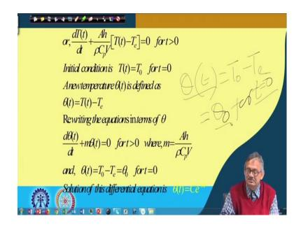
So, if this be true the we can write that as we have said the initial condition is  $\theta_t$  is equal to  $T_t$ - $T_e$  which is equal to  $\theta_0$  and this is valid for t time is equal to 0; that is why it is called initial condition at time t is equal to 0, 'right'. So, at time t is equal to 0,  $\theta_t$  is equal to  $\theta_0$  and defined as  $T_t$ - $T_e$ , 'right'.
