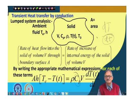
So,  $mC_p\Delta T$  and this  $\Delta T$ , is a function of time, 'right' that is why we write dT/dt that is del del T of t, that is, rate of change of temperature with respect to time. So, this equation we can solve that the governing equation which we have said rate of heat flow into the solid of volume V through the boundary surface A must be equal to the rate of increase of internal energy.
