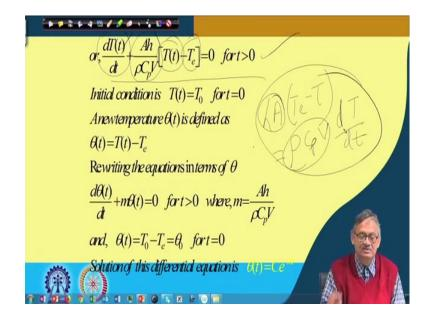
So, once we have this the solution of heat can be written as  $\frac{dT(t)}{dt} + \frac{Ah}{\rho C_{\nu}V} \left[ T(t) - T_e \right] = 0 \quad for \ t > 0$
