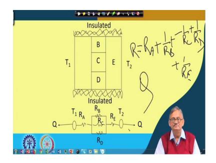
So,  $R_A$  plus, total R will be  $R_A+1$  / $R_B+R_C$  +1  $R_D+1/R_E$ , 'right' which we did in the previous one also. So, ones  $R_A$ ,  $R_B$ ,  $R_C$ ,  $R_D$ ,  $R_E$  are known we find out that value of Q, 'right', so this is another example of combination.
