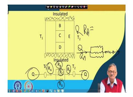
So, we know A; we know  $R_B$ ,  $R_C$ ,  $R_D$ ,  $R_E$ , then we can easily find out Q that taking that  $R_A$  is in  $R_A$  is there. So, then we have 3 parallel resistances,  $R_B$ ,  $R_C$ ,  $R_D$ , 'right', which 3 are then going through  $R_E$  and then going out as Q, 'right', this is as Q.
