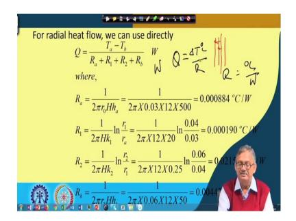
$$Q = \frac{T_a - T_b}{R_a + R_1 + R_2 + R_b} \quad W$$
