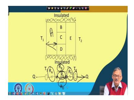
So, that gives us  $R_A$  and this again going through all these 3 one is  $R_B$  and these  $R_C$  and another is  $R_D$  there are in parallel. Then all these 3 parallel are coming to this point, from this point and then going to the  $R_E$  and to the temperature  $T_2$  and then going out as Q, 'right'.
