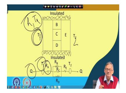
So, Q quantity of heat is coming to the point  $T_1$ , which the resistance of  $R_A$  corresponding to this  $T_1$ , because this  $T_1$  can we corresponding to 1  $h_1$  and another  $T_a$  which will give us  $R_A$ . Then it has come to that point and that if it is assume that this is a constant temperature boundary, this is also a constant temperature boundary that this boundary is giving first resistance of this which is  $R_A$ , so this is the material A, 'right',
