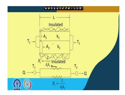
Or insulation can be also like this, it is  $A_1$ ,  $k_1$ ,  $A_2$ ,  $k_2$ , L is constant. So, this is maintain that  $T_1$  this is maintain that  $T_2$ , 'right'. So, similar this if it is then, we know that 1/R, equal to  $A_1k_1/L + A_2k_2/L$ , 'right'. So, this means  $A_1$  given 0.3, and L is 0.6,  $k_1$  given 25 and L 0.6,  $A_2$  given 0.5,  $k_2$  given 20, L same 0.6. So, this becomes 29.16 that is 1/R.
