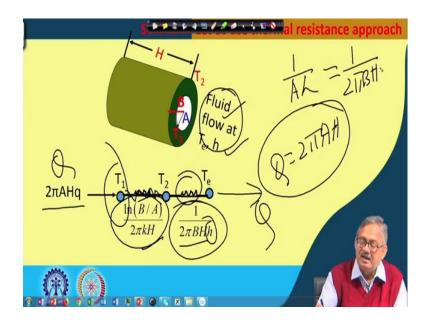
So, inner radius is that; so, that is what we are supplying Q, 'right'. The same Q is going out through the other side and the inner temperature is  $T_1$ , 'right'. So, there is a resistance and this resistance is equivalent to  $\ln(B/A)/2\pi kH$  which we have seen earlier and the outer surface is at the boundary. It is a fluid at temperature  $T_e$  with a heat transfer coefficient of H, 'right'.
