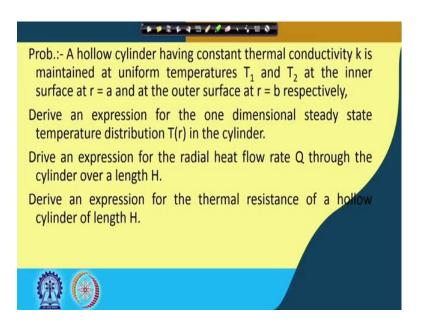
A hollow cylinder having constant thermal conductivity k is maintained at uniform temperature  $T_1$  and  $T_2$ . This we have done. This solution of it we have done and we have seen that the area is coming Log mean area, 'right' and the solution it came to be like this, 'right'.
