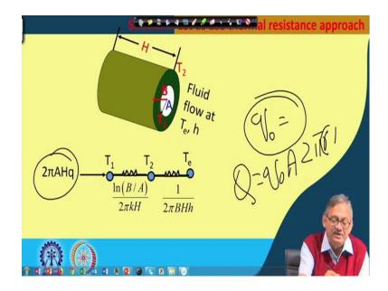
So, heat flux is coming we are given  $q_0$  equal to some value afterwards ok. Now,  $q_0$  is coming; so, Q is equal to  $q_0$  times area, 'right'. So, area is here  $2\pi rH$  'right' or  $2\pi$  yes, in this case it is A; instead of r, we are writing A, because our given is Q is equal to  $2\pi A$  into H; H is the length, 'right'. So, our radius given is A.
