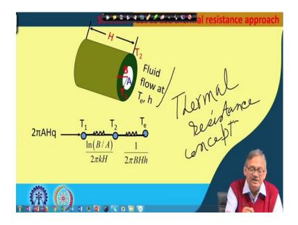
So, if we see this we can make this like that. As you see that we have taken a cylinder, this is a hollow cylinder, 'right'. This white portion is saying to be hollow, 'right' and it has a radius of B and also a radius of A and this surface is  $T_1$  at this inner radius and
