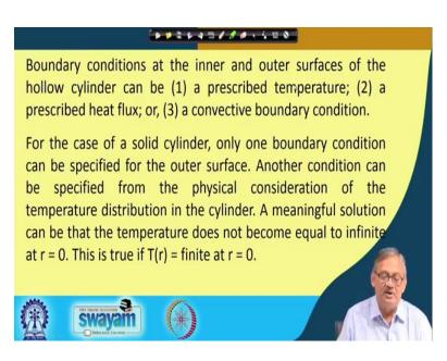
So, if that is the case then we can now, write that the boundary condition at this inner and outer surfaces of the hollow cylinder can be one either prescribed temperature boundary condition; or a prescribed heat flux boundary condition; or a convective boundary condition, 'right'. Either of this any of two of these three, I in combination or singly that can be the typical case, 'right'.
