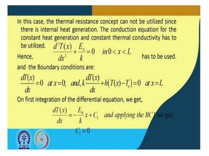
So, in this case the thermal resistance concept cannot be utilized, because there is internal energy generation. The condition or the conduction equation for the constant heat flux, or the constant not heat flux, for the constant heat generation, and constant thermal conductivity has to be utilized. And, now we start with that where we ended with you remember we said that the here it is steady state.
