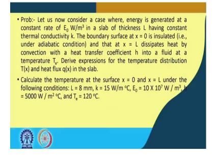
So, we come to this that problem. Let us know how consider a case where energy is generated at constant rate of  $E_0$  W/m<sup>3</sup> in a slab of thickness L having constant thermal conductivity k.
