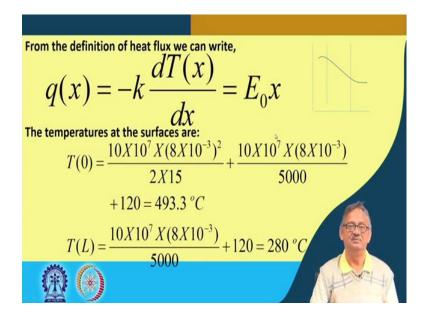
So, this is for energy generation and this is for the heat transfer coefficient. So, we can write that  $q(x) = -k \frac{dT(x)}{dx} = E_0 x$ . So, we have the solution we have found out the temperature distribution T(x) and also you have found out the q(x) at any x which is  $E_0 x$ , 'right'. Now, we can solve easily and find out the temperatures at x equal to 0 and that x as to L
