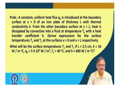
So, we let us take another problem a constant uniform heat flux  $q_0$  is introduced at the boundary surface at x is equal to 0 of an iron plate of thickness L with thermal conductivity k. From the other boundary surface at x is equal to L, heat is dissipated by convection into a fluid at temperature T<sub>e</sub> with the heat transfer coefficient h.
