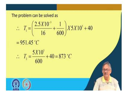
So, if we have already found out  $T_1$  and  $T_2$  we can easily now calculate the numerical values, because all others are given. So,
