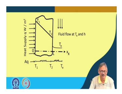
Here is that pictorially we can you can write it this is the iron slab and one side is heat supply by q we what so, much watt per meter square this is that, 'right'.
