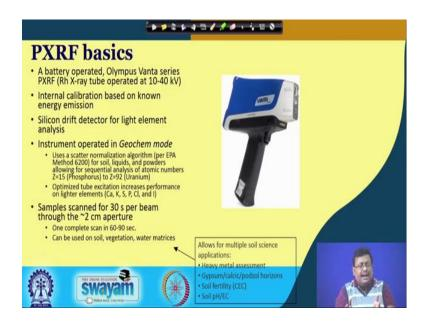
So, this is basically battery operated this an model Vanta which is one of the advanced model produced by Olympus company. And this is this x-ray, this contains a rhodium x-ray tube which operated at 10 to 40 kilo electron volt and then the internal calibration based on known energy emission and obviously, it has got a silicon drift detector for light elemental analysis.
