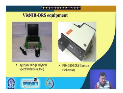
So, let us see some equipments for VisNIR - DRS spectro radiometer. So, you can see there are two equipments: one is called AgriSpec DRS by analytical spectral devices of USA and this is spectral evolution 3500 DRS. So, it is actually PSR 3500. So, please correct it is PSR 3500 or so, these are two important instruments nowadays available for VisNIR - DRS measurement. So, let us go ahead and see what is the internal config of these two instruments.
