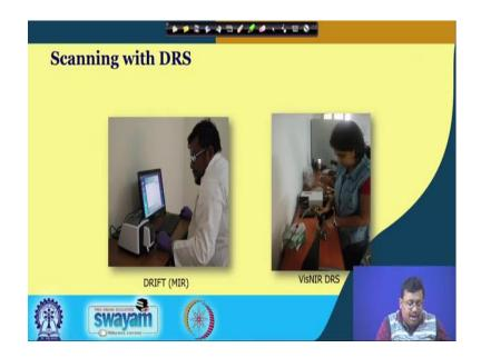
So, we collected the samples and then we scan using these two techniques; one is the mid infrared spectrometer we call a drift or diffuse reflectance infrared fourier transform technique another is visible near infrared diffuse reflectance spectroscopy.
