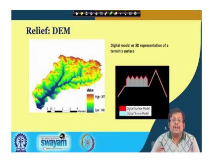
So, not only the soil features also you can use for identifying remote sensing you can use for you know creating the DEMs and the DEM is basically Digital Elevation Model which is a 3D representation of the terrain surface. It is basically save in terms of rasters or gridded cells and this gridded cells are basically containing different numbers or different elevations values which we can see in you know in the form of DEM.
