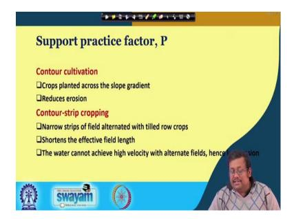
So; obviously, the contour cultivation; obviously, crops are planted across the slope gradient to reduce the erosion. And in the contour strip croppings, narrow strips of field alternate with tilled row crops and it basically shortage the effective field length and the water cannot achieve high velocity with alternate fields hence less erosion. So, these are the, features of contour cultivation as well as contour strip cropping.
