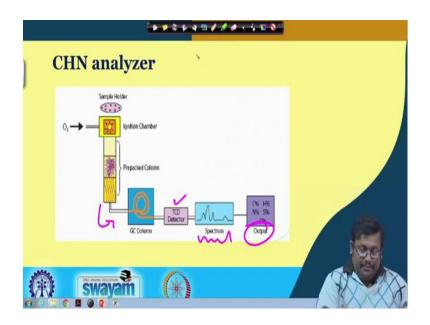
So, the so the working principle of CHN analyser in a there is a sample holder. And there is an ignition chamber, we incorporate oxygen through it. So, the sample is injected here there is a pre-packed column.
