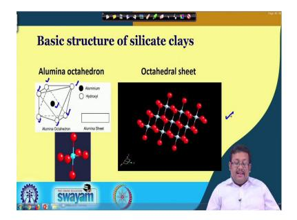
So, if you go to the next slide let us see what is another building block. So, another building block in soil is the aluminium octahedra and this aluminium octahedron the individual aluminium octahedron is basically made of the central aluminium and which is surrounded by 6 hydroxyl you know hydroxyl anions or hydroxyl groups making a octahedral structure.
