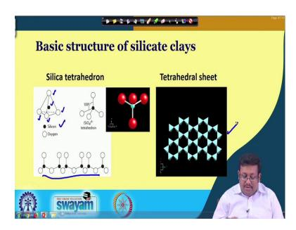
So, let us focus on silica tetrahedra and their related structures. So, as we can see as I have discussed that this is the silica tetrahedra which is composed of four equidistantly placed oxygen atom and in the inside there is a silica atom.
